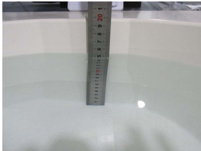
Fig.17 Body Liquid of 835MHz(15cm)
