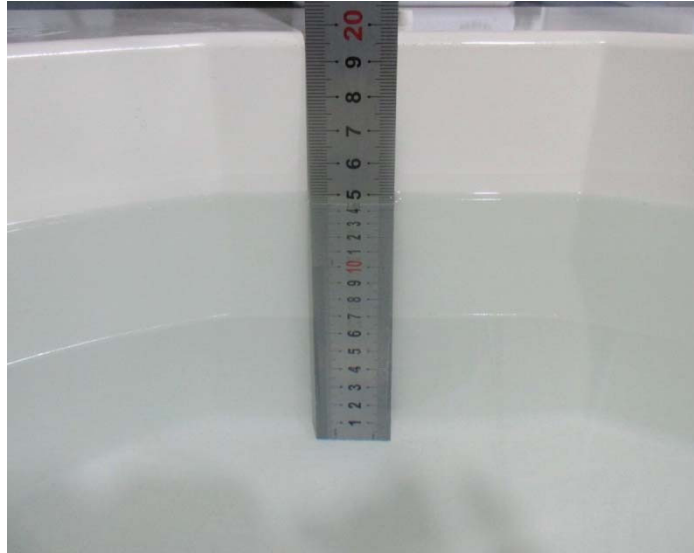
Fig.18 Body Liquid of 1900MHz(15cm)
