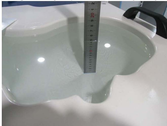
Fig.19 Head Liquid of 2450MHz(15cm)
