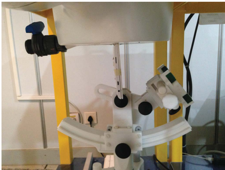
Fig.13 Tablet Edge B (Back upside,0mm separation)
