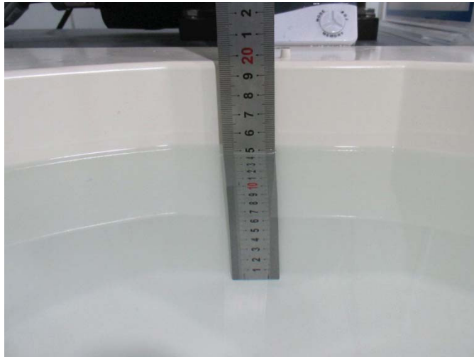
Fig.16 Head Liquid of 835MHz(15cm)
