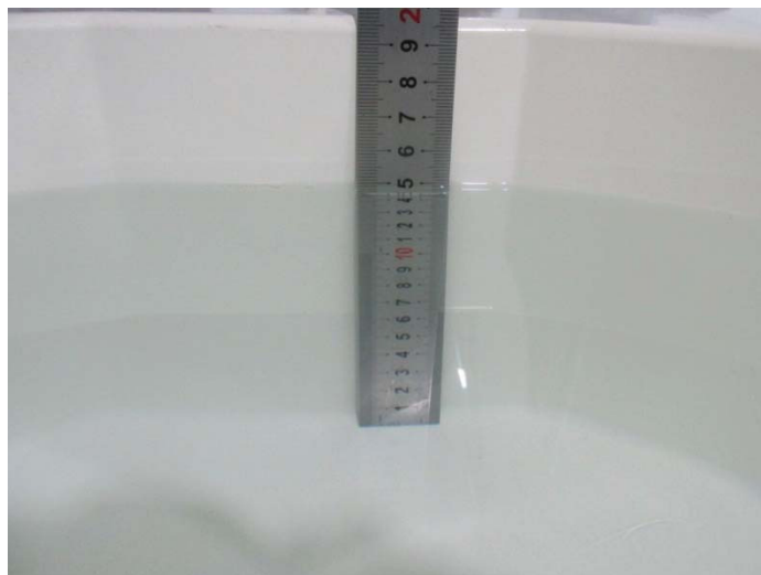
Fig.17 Body Liquid of 835MHz(15cm)
