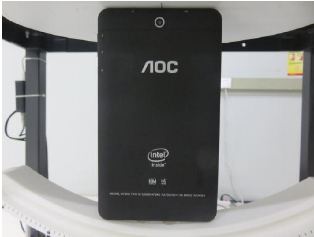
0mm body-worn Top Side Setup Photo(hotspot)
