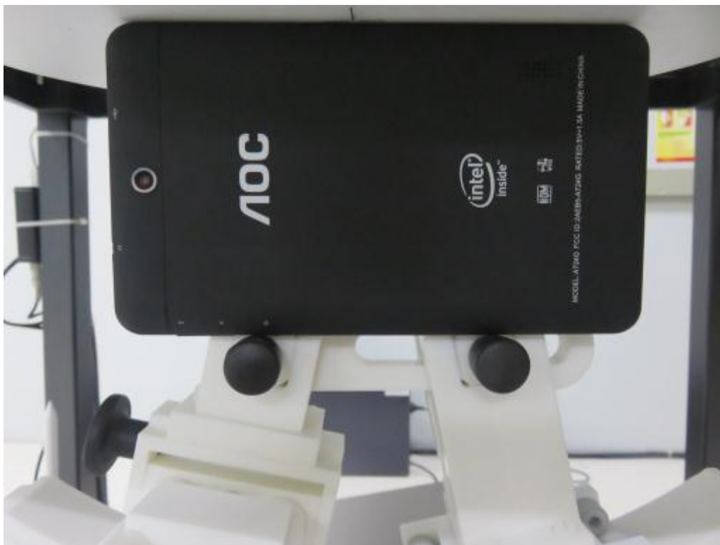
0mm body-worn Left Side Setup Photo(hotspot)
