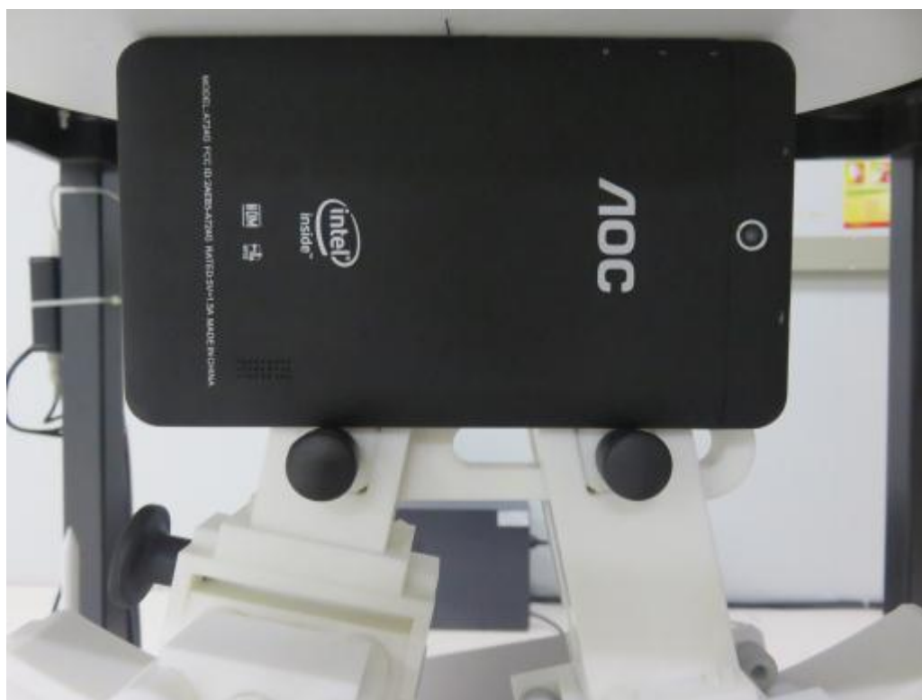
0mm body-worn Left Side Setup Photo(hotspot)
