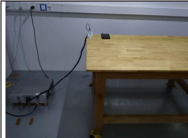
Conducted Emissions Test Setup – Front View
