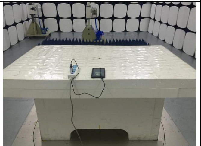
Radiated Emissions Test Setup Above 1GHz
