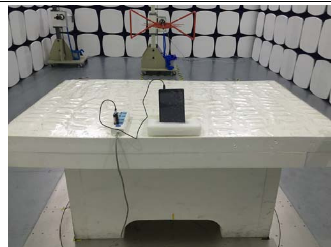
Conducted Emissions Test Setup Front View
