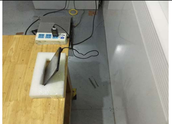
Conducted Emissions Test Setup Side View
