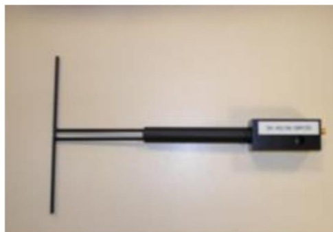
Figure 1 – Satimo COMOSAR Validation Dipole
