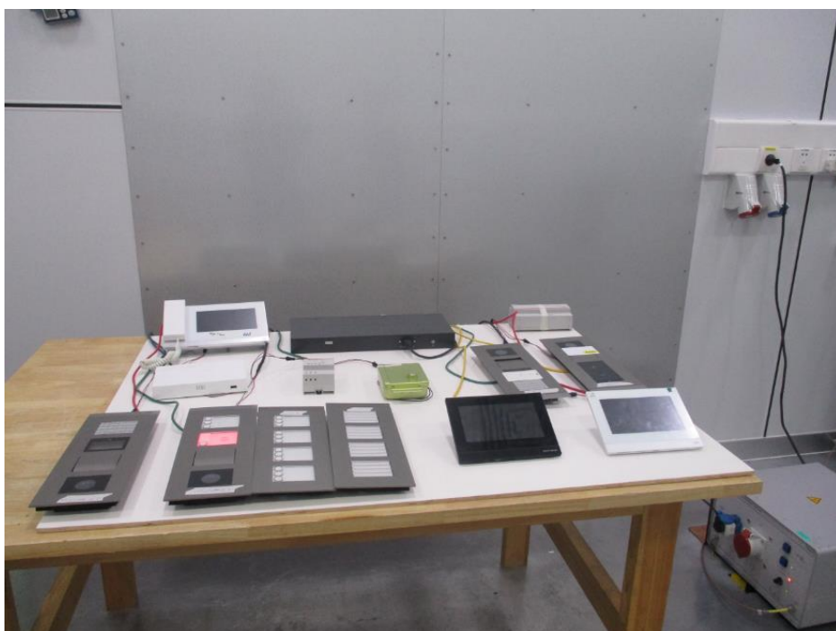
Setup photo of conducted emission (150KHz-30MHz)
