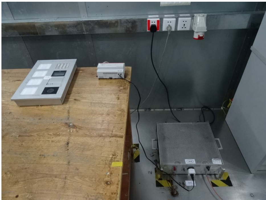
Setup photo of conducted emission (150KHz-30MHz)
