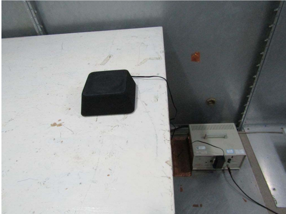
Measurement of Conducted Emission Test Set Up
