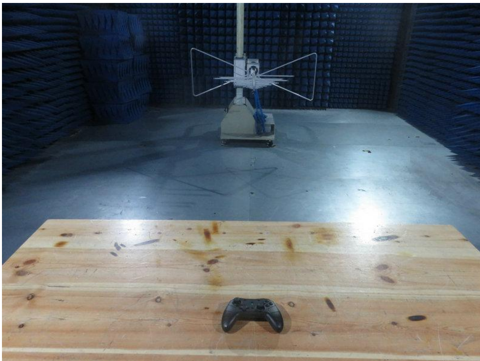
Photo of Radiation Emission Test
