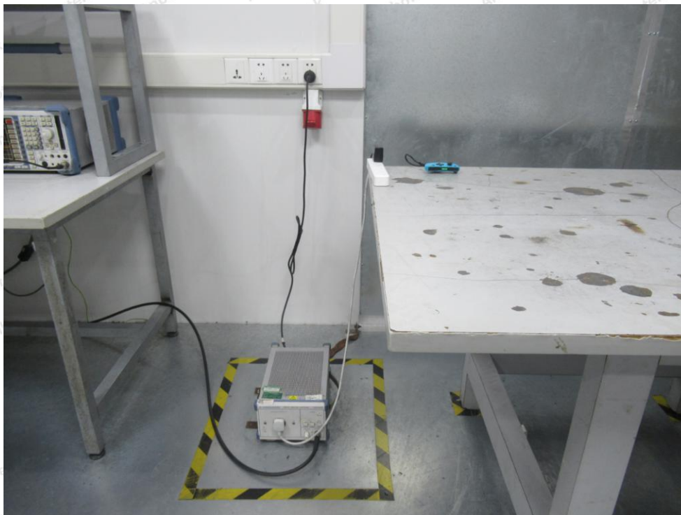
Photo of Conducted Emission Measurement
