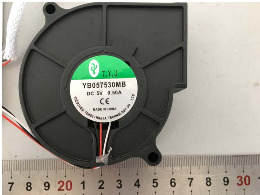
EUT –Fan View
