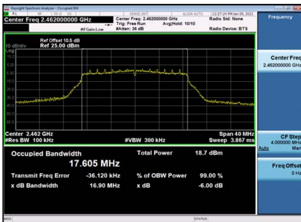
6dB Bandwidth-802.11n(HT20),2462MHz
