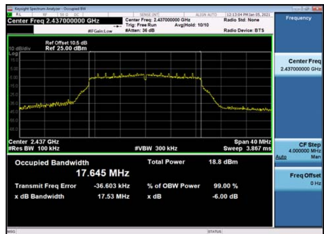
6dB Bandwidth-802.11n(HT20),2437MHz
