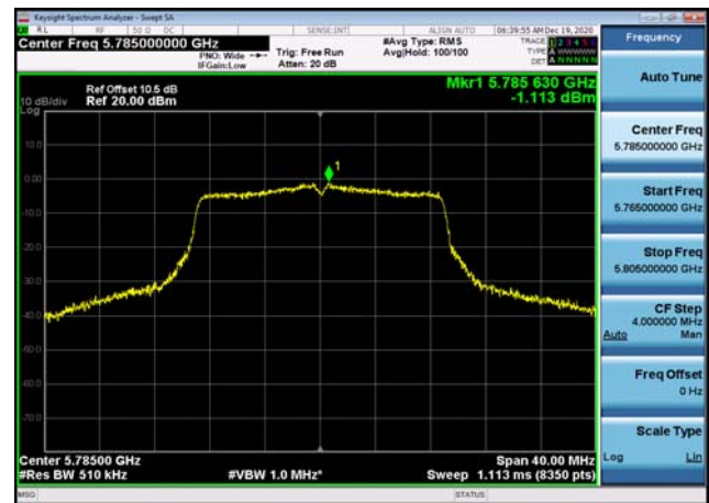
U-NII-3 Power spectral density-802.11 ac(20MHz),5785MHz
