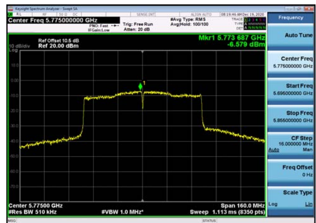
U-NII-3 Power spectral density-802.11 ac(80MHz),5775MHz
