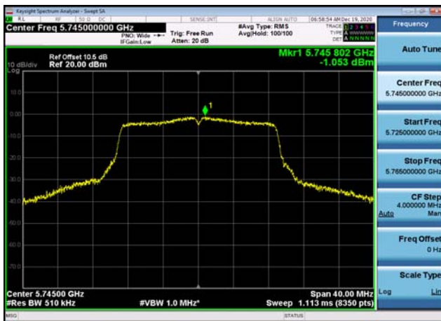
U-NII-3 Power spectral density-802.11 ac(20MHz),5745MHz
