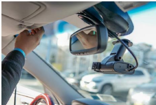
3 - Route the camera harness across the headliner
