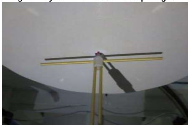
Fig.10.2 Photo of Dipole setup
