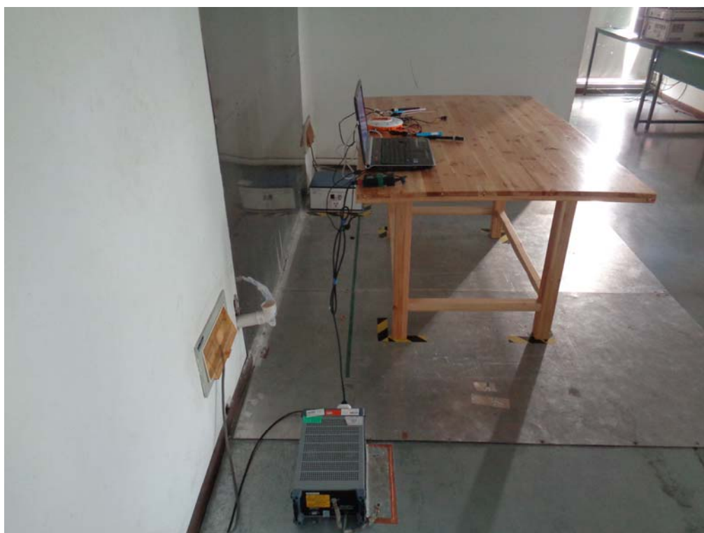
Conducted Emissions Setup Side View
