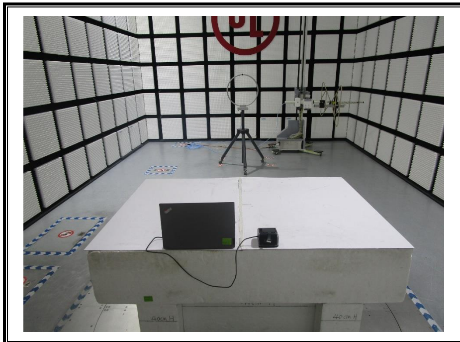
RADIATED RF MEASUREMENT SETUP (Below 30MHz)
