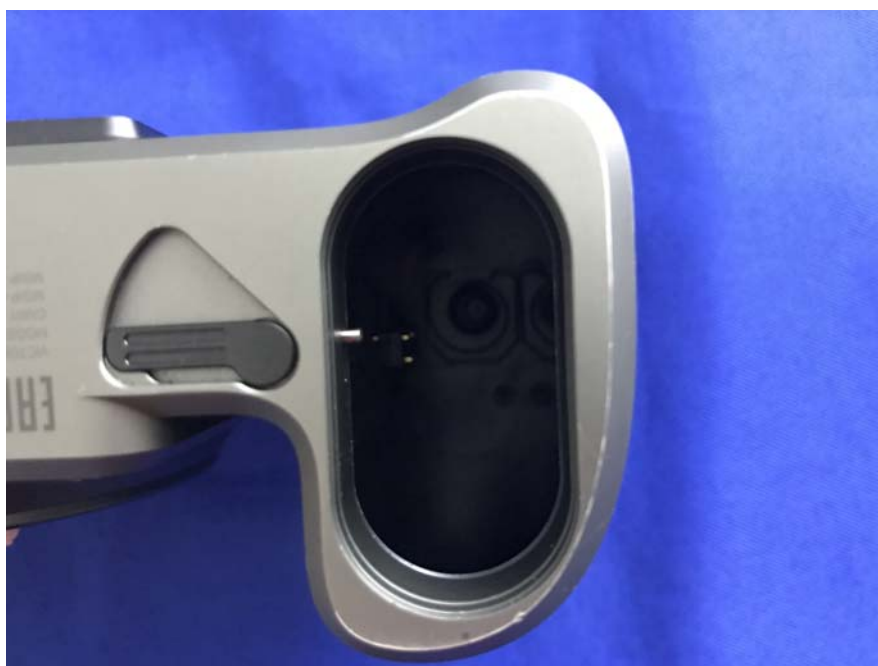
EUT – Battery Compartment View
