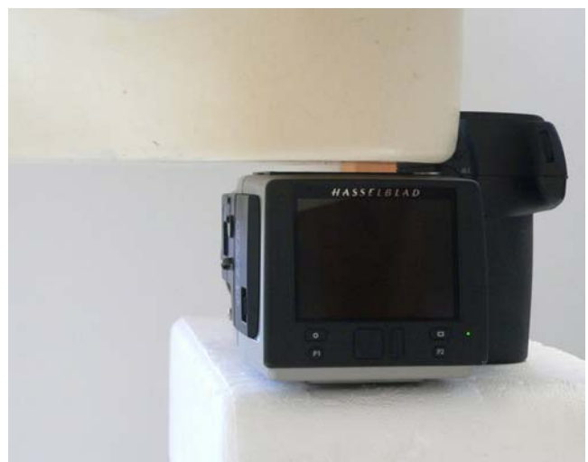
Fig. 15: Top side towards the phantom, view finder detached, 5 mm distance.
