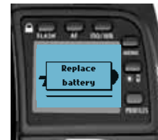
Exhausted battery warning
