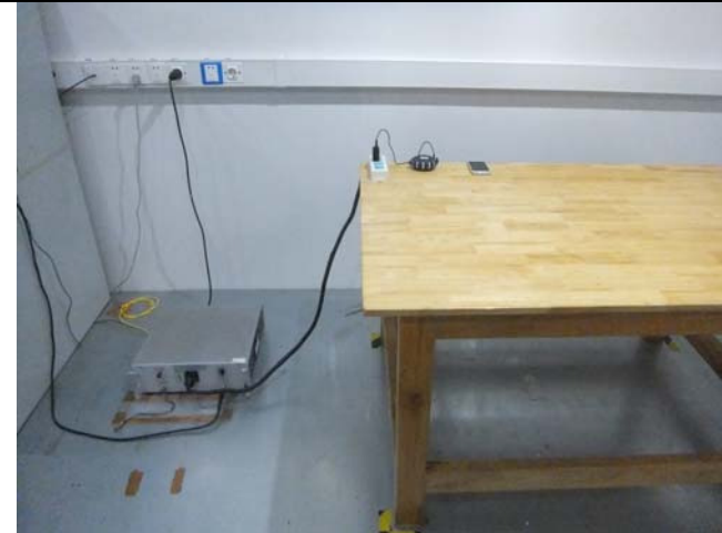
Conducted Emissions Test Setup Front View
