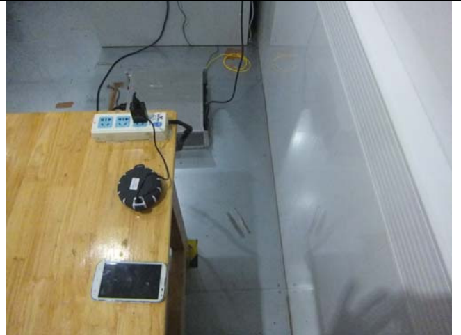
Conducted Emissions Test Setup Side View
