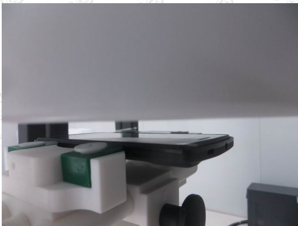
10mm body-worn Front Side Setup Photo(hotspot)
