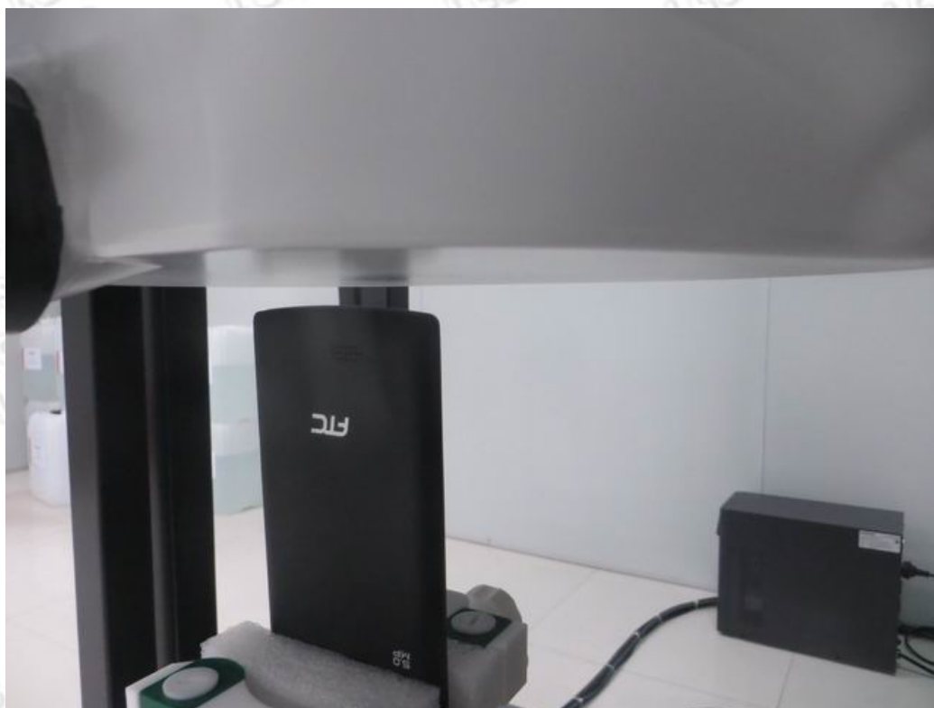
10mm body-worn Bottom Side Setup Photo(hotspot)
