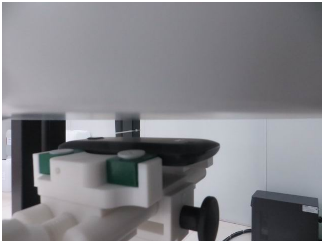
15mm body-worn Back Side Setup Photo
