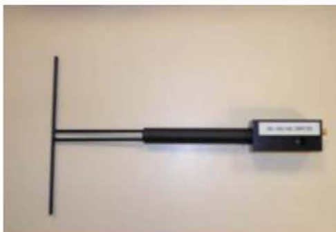
Figure 1 – Satimo COMOSAR Validation Dipole
