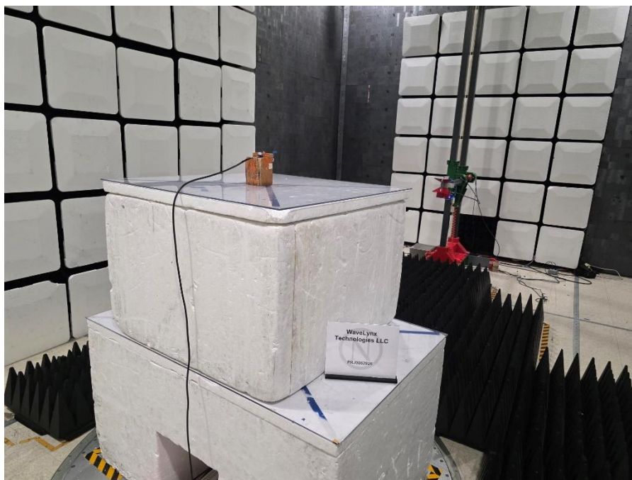
Figure 4 - Radiated emissions above 1 GHz (1 – 18 GHz), rear view.
