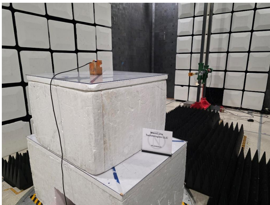
Figure 6 - Radiated emissions above 1 GHz (18 – 26.5 GHz), rear view.
