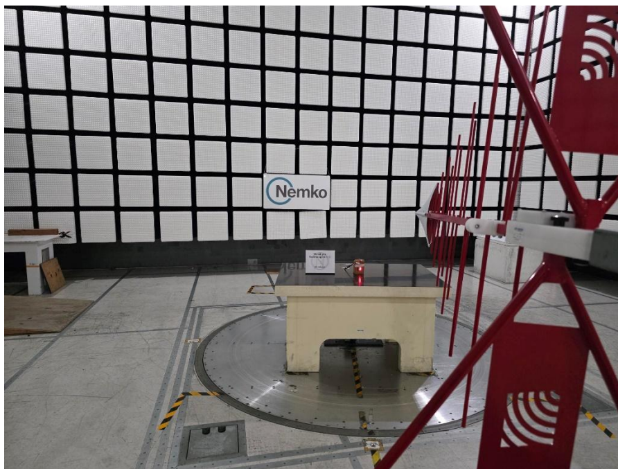
Figure 1 - Radiated emissions below 1 GHz (0.03 – 1 GHz), front view.
