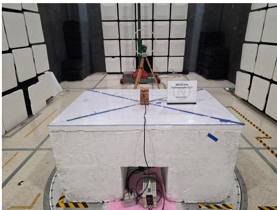
Figure 2 - Radiated emissions below 30 MHz, 0 Degree, rear view
