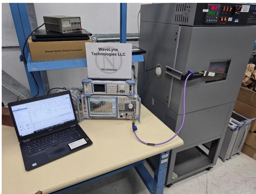
Figure 8 – Test setup, frequency stability – Varying Temperature
