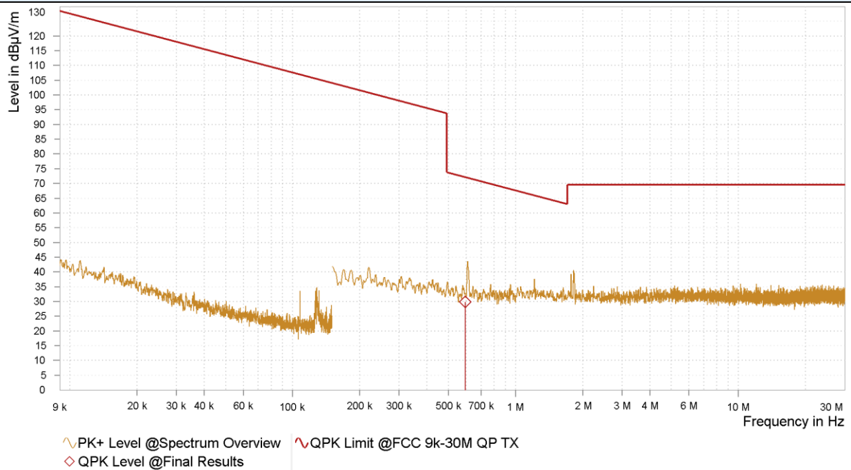
Radiated Spurious Emission 9 kHz – 30 MHz (Antenna Position 180°): 2.4GHz ISM Mid
