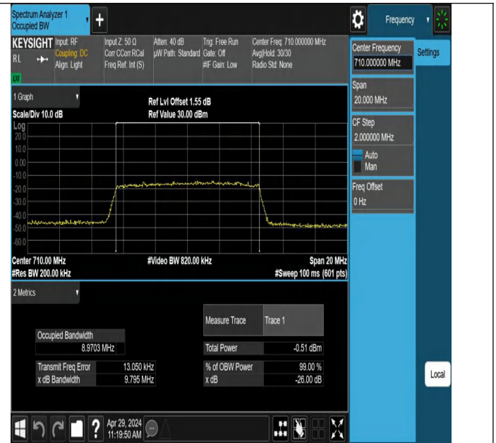
Band17-10MHz-64QAM-23790-50RB#0-PASS
