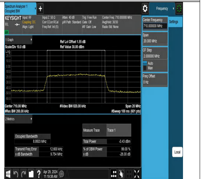
Band17-10MHz-16QAM-23790-50RB#0-PASS
