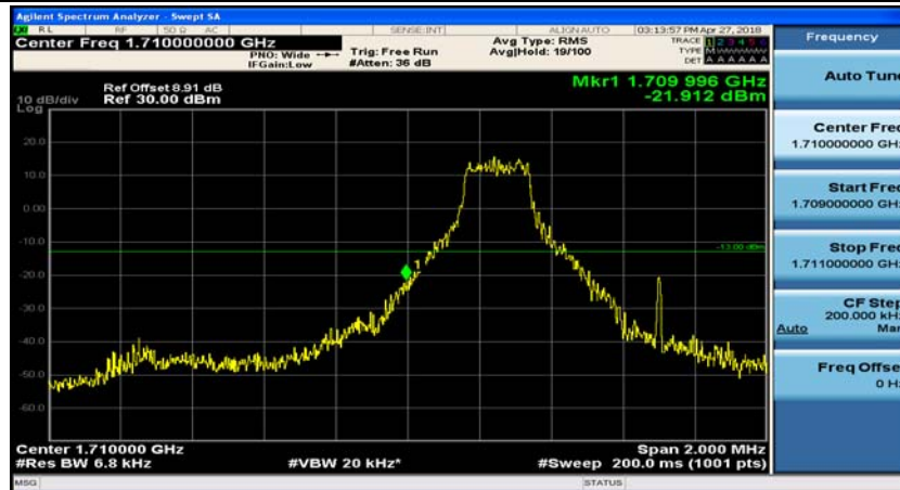
(Channel Bandwidth: 1.4 MHz)_LCH_QPSK_1RB#3
