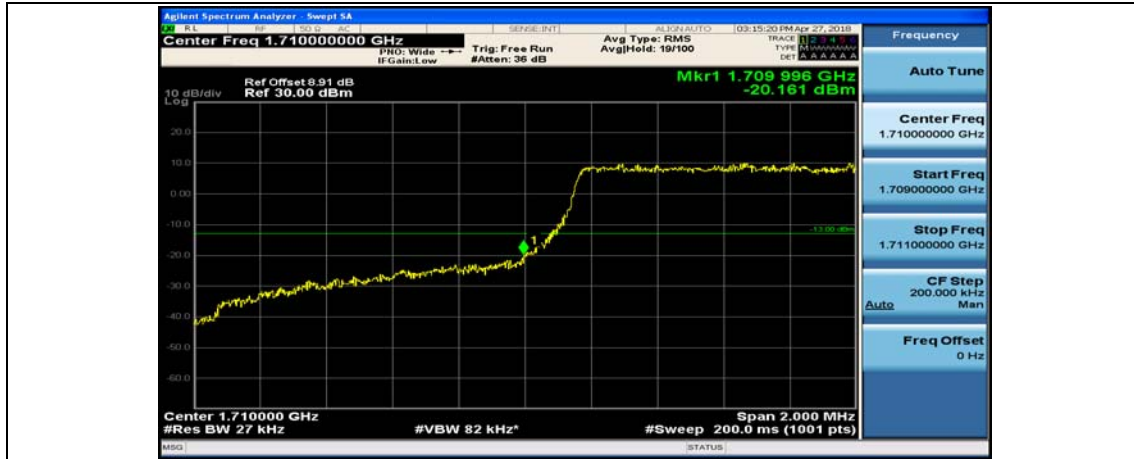
(Channel Bandwidth: 1.4 MHz)_HCH_QPSK_1RB#0
