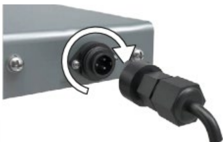
Connect Power Cable at Rear Side
