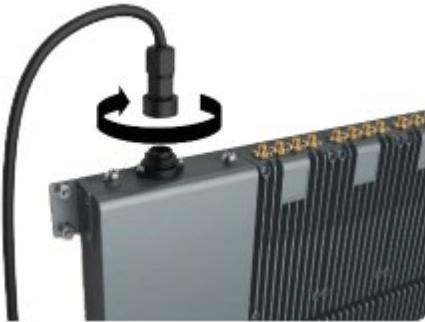
Connect power cable at the rear of the unit
