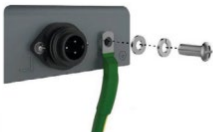
Connect Ground Cable at Rear Side
