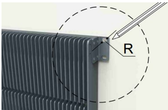
Marking the Position of Mounting Holes
