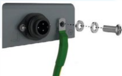
Connect Ground Cable at Rear Side
