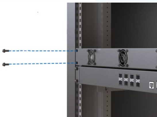
Fix Fan with Screws
