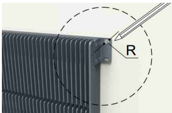
Marking the Position of Mounting Holes
