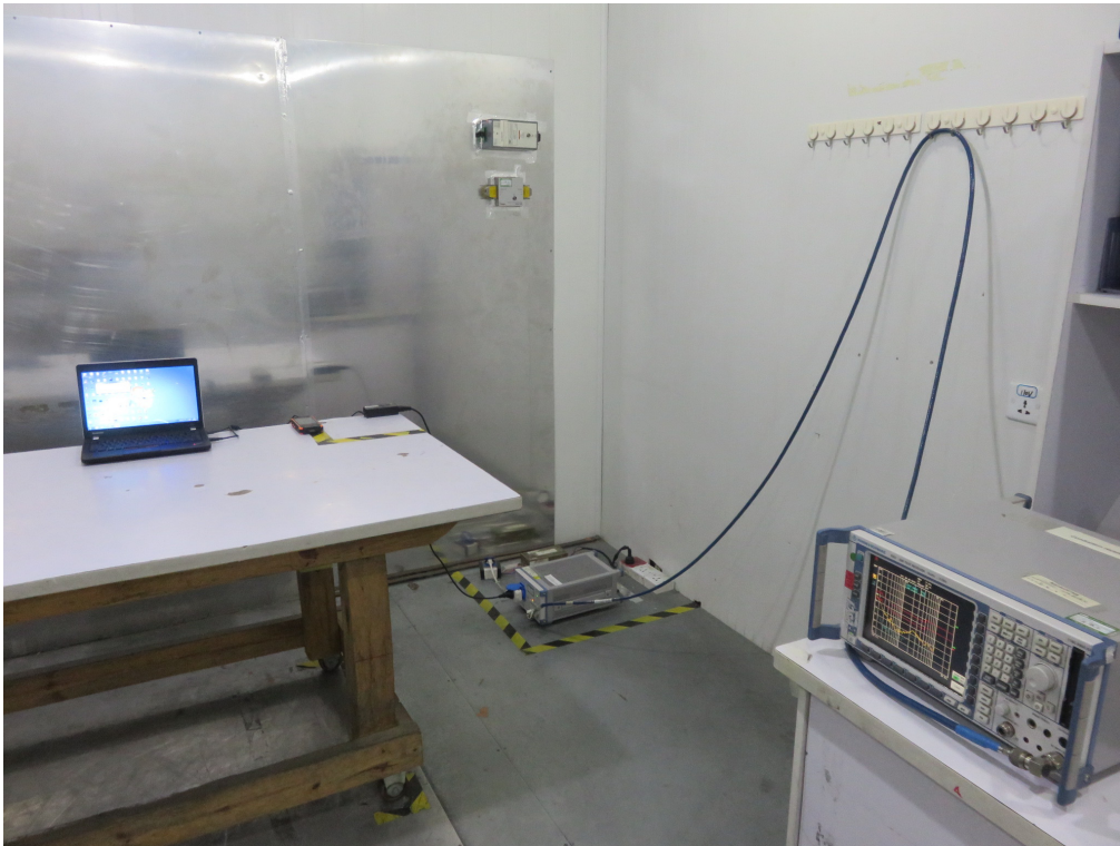
FCC RADIATED EMISSION TEST SETUP
