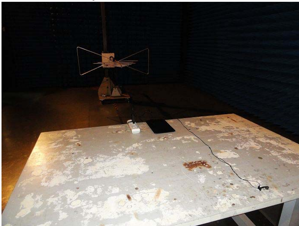
Radiated Emission Test Setup:
