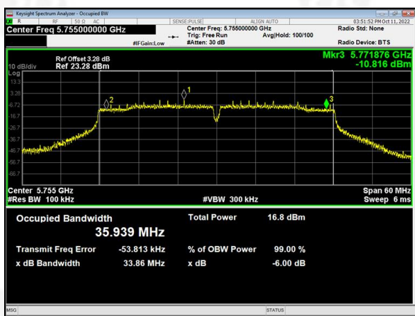
(802.11 ac40) 6dB Bandwidth plot on channel 159
