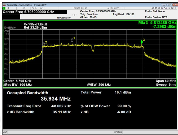
(802.11 ac40) 6dB Bandwidth plot on channel 159
