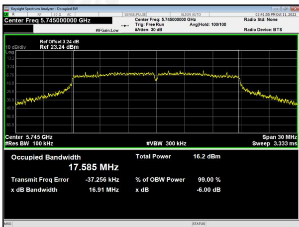
(802.11ac20) 6dB Bandwidth plot on channel 157
