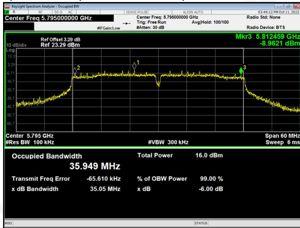
(802.11 n40) 6dB Bandwidth plot on channel 159
