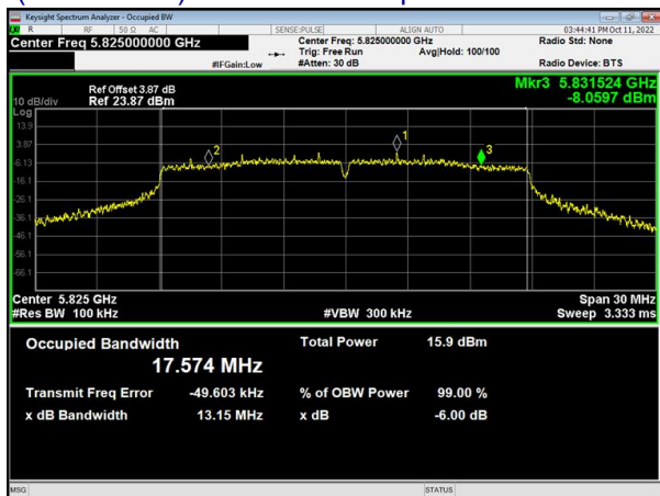
(802.11ac20) 6dB Bandwidth plot on channel 165
