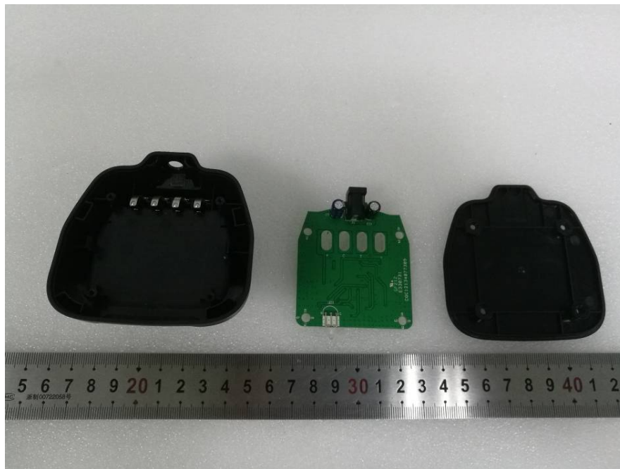
EUT(Charger) – Cover off View
