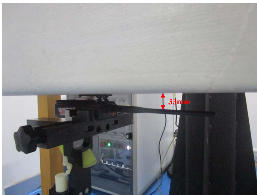
Body Worn Back Setup Photo(0mm)
