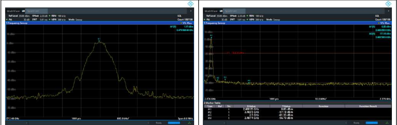
GFSK: Band Edge, Right Side
