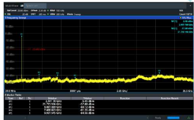
8DPSK on Channel 39
