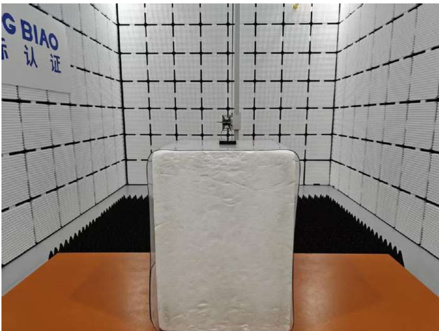
Radiated Emission Above 1GHz
