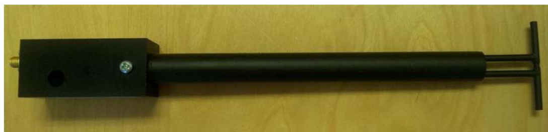
Figure 1 – MVG COMOSAR Validation Dipole
