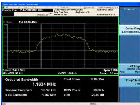
20dB Bandwidth plot on channel 78 (3Mbps)
