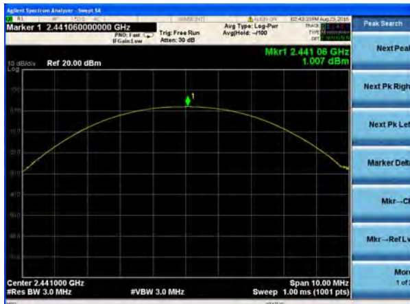
Peak output Power plot on channel 78 (2Mbps)
