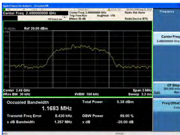
20dB Bandwidth plot on channel 78 (3Mbps)
