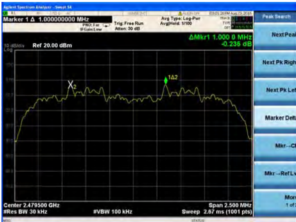
(2Mbps) Channel Separation plot on channel 77-78
