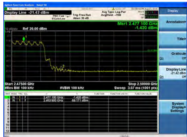
BDR mode (8DPSK): Band Edge-High Channel (Hopping Mode)
