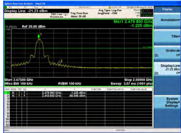
BDR mode (8DPSK): Band Edge-High Channel (Hopping Mode)
