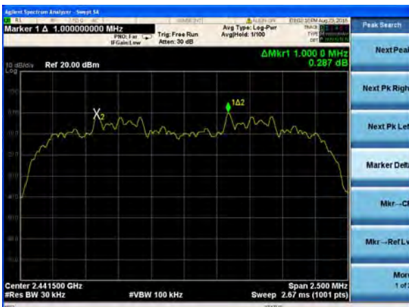
(2Mbps) Channel Separation plot on channel 39-40
