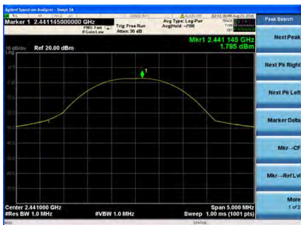
Peak output Power plot on channel 78 (1Mbps)
