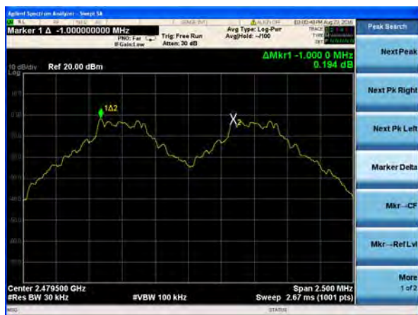
(1Mbps) Channel Separation plot on channel 77-78
