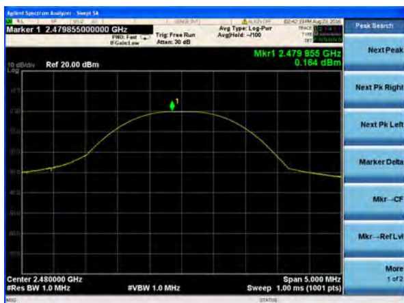
Peak output Power plot on channel 78 (1Mbps)
