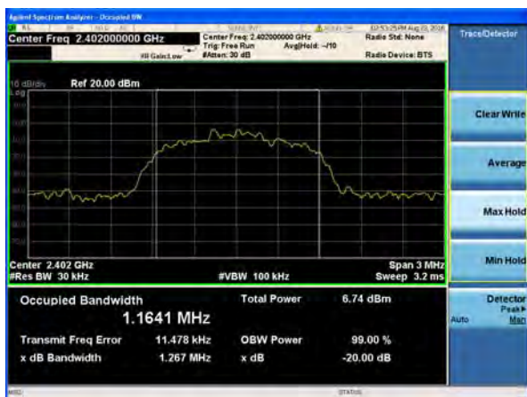
20dB Bandwidth plot on channel 00 (3Mbps)
