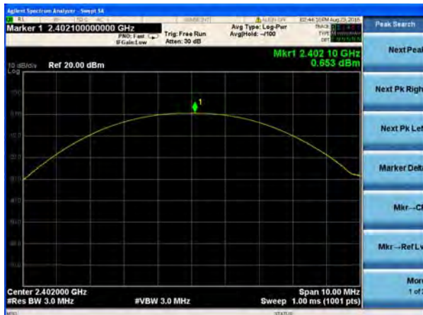
Peak output Power plot on channel 39 (2Mbps)
