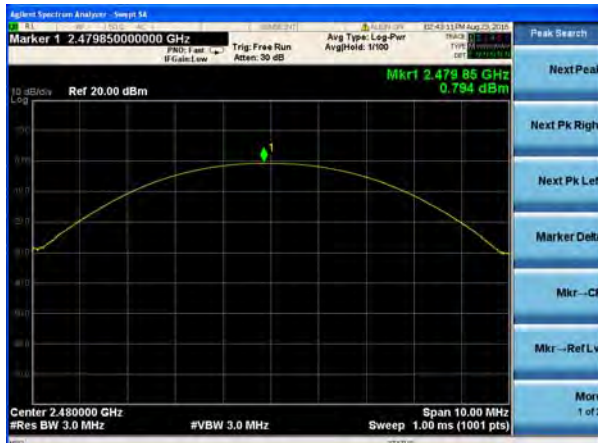
Peak output Power plot on channel 78 (2Mbps)
