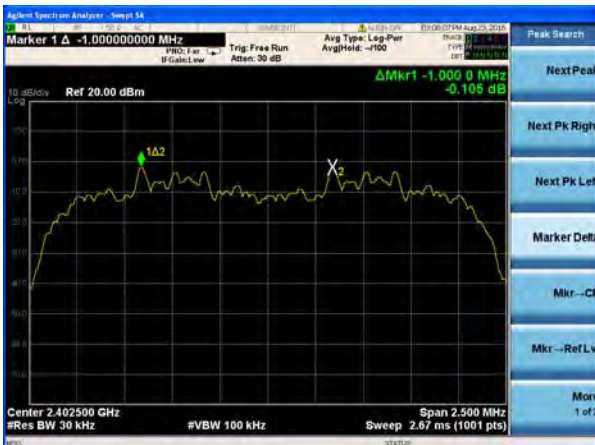
(2Mbps) Channel Separation plot on channel 39-40
