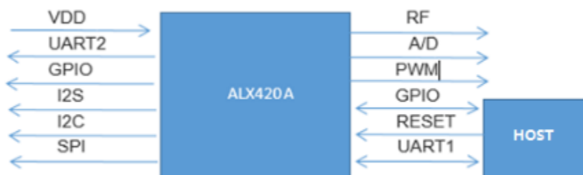
Figure 13 - Hardware Design with external MCU
