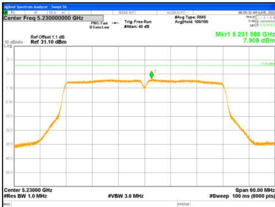
Figure 62: FCC Correlated Power Spectral Density-5230 MHz-802.11n-HT40-MCS0-Ch1
