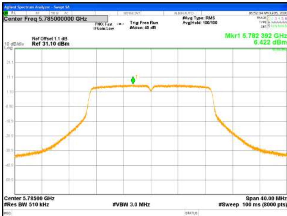
Figure 60: Correlated Power Spectral Density-5785 MHz-802.11n-HT20-MCS0-Ch1
