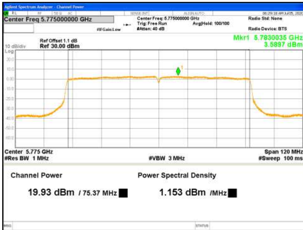
Figure 33: Correlated Max Conducted Power-5775 MHz-802.11ac-VHT80-MCS0-Ch0
