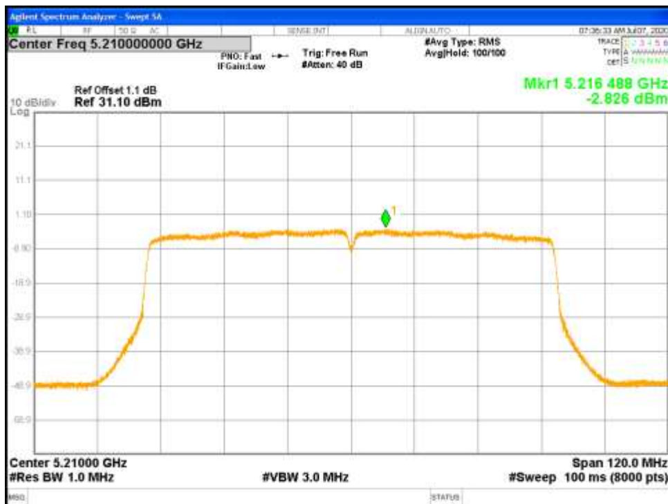
Figure 70: RSS Correlated Power Spectral Density-5210 MHz-802.11ac-VHT80-MCS0-Ch1
