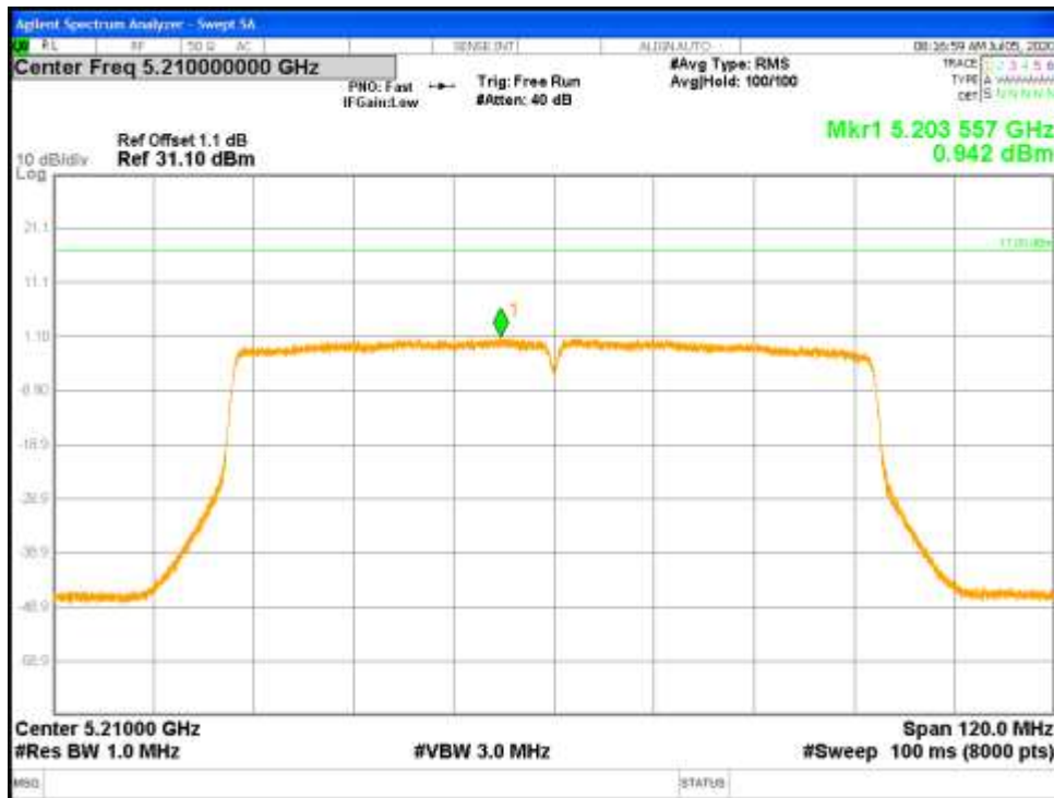
Figure 67: FCC Correlated Power Spectral Density-5210 MHz-802.11ac-VHT80-MCS0-Ch0
