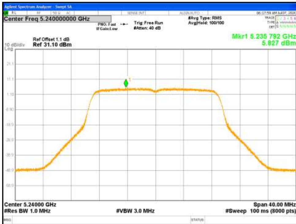
Figure 47: RSS Uncorrelated Power Spectral Density-5240 MHz-802.11n-HT20-MCS0-Ch0
