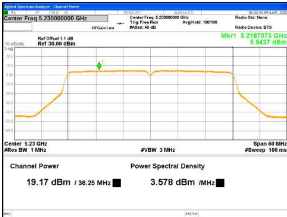
Figure 12: RSS Uncorrelated Max Conducted Power-5230 MHz-802.11n-HT40-MCS0-Ch0
