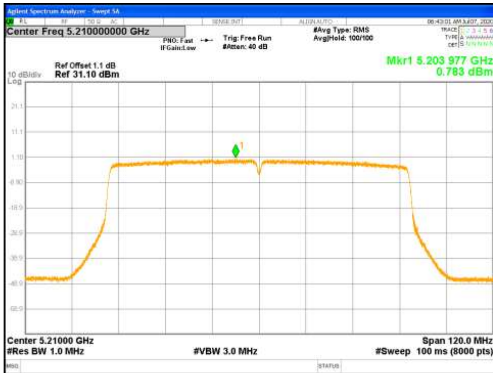
Figure 53: RSS Uncorrelated Power Spectral Density-5210 MHz-802.11ac-VHT80-MCS0-Ch0
