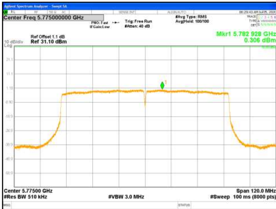
Figure 71: Correlated Power Spectral Density-5775 MHz-802.11ac-VHT80-MCS0-Ch0
