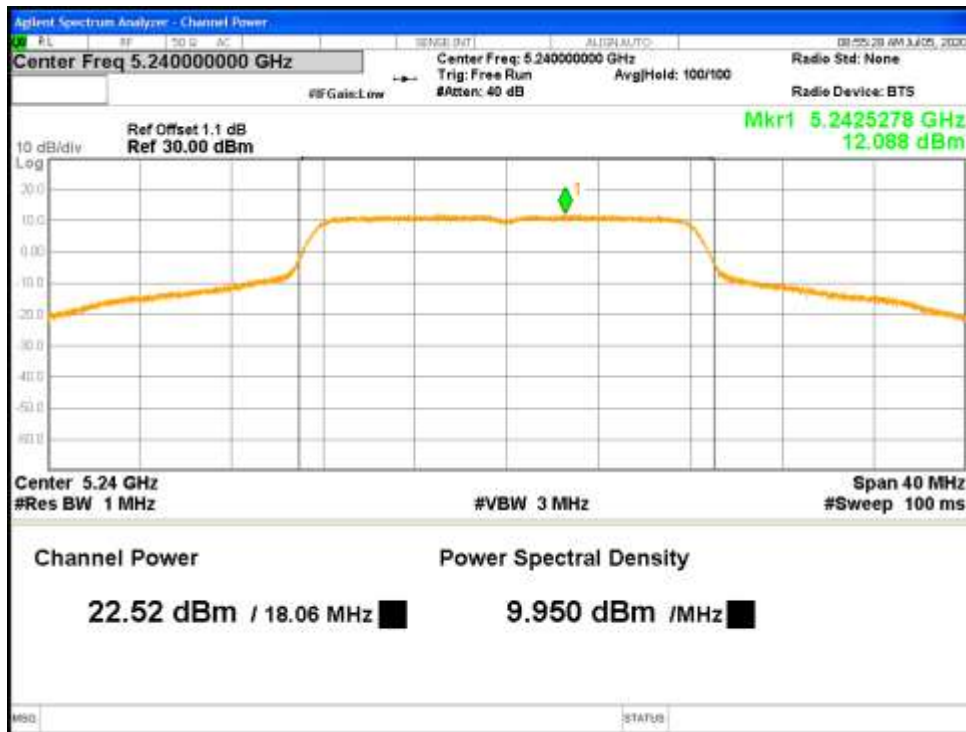
Figure 5: FCC Uncorrelated Max Conducted Power-5240 MHz-802.11a-6 Mbps-Ch0
