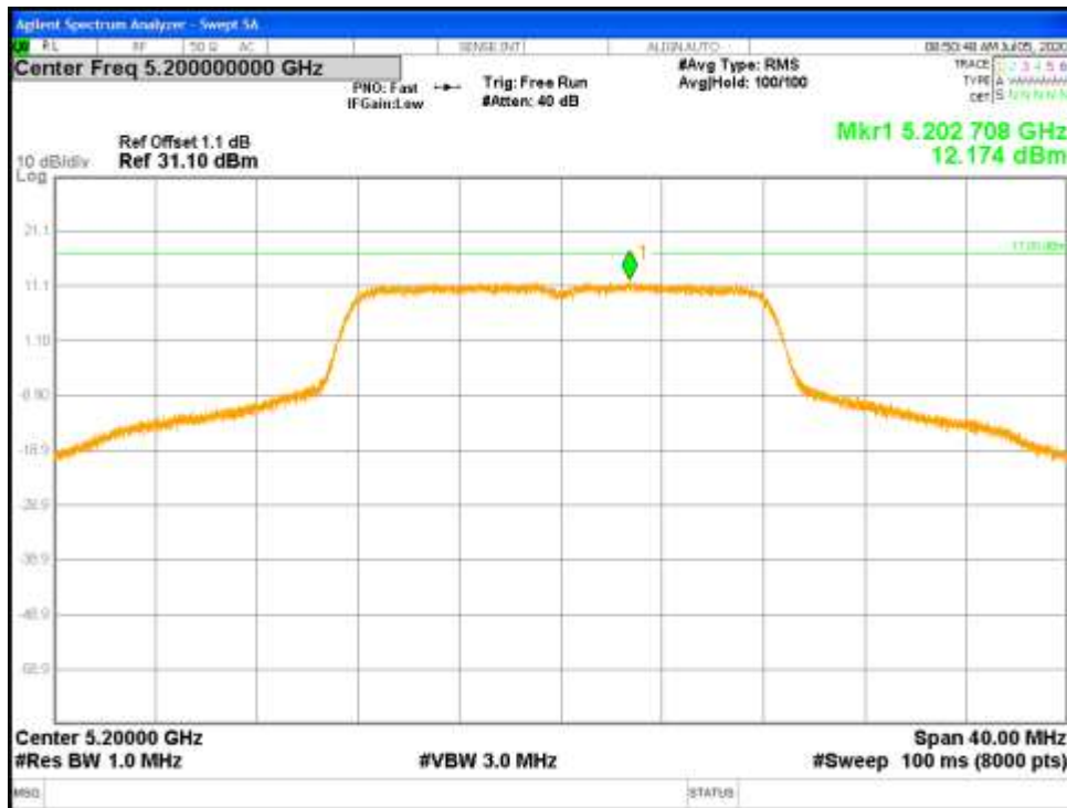
Figure 43: FCC Uncorrelated Power Spectral Density-5200 MHz-802.11a-6 Mbps-Ch0
