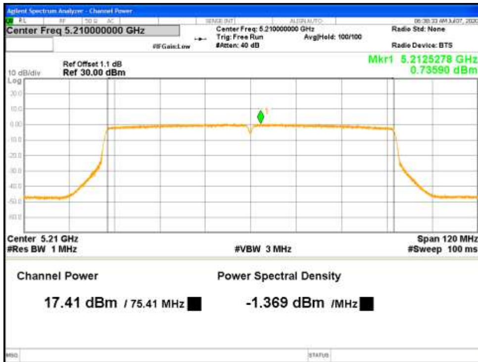
Figure 15: RSS Uncorrelated Max Conducted Power-5210 MHz-802.11ac-VHT80-MCS0-Ch1
