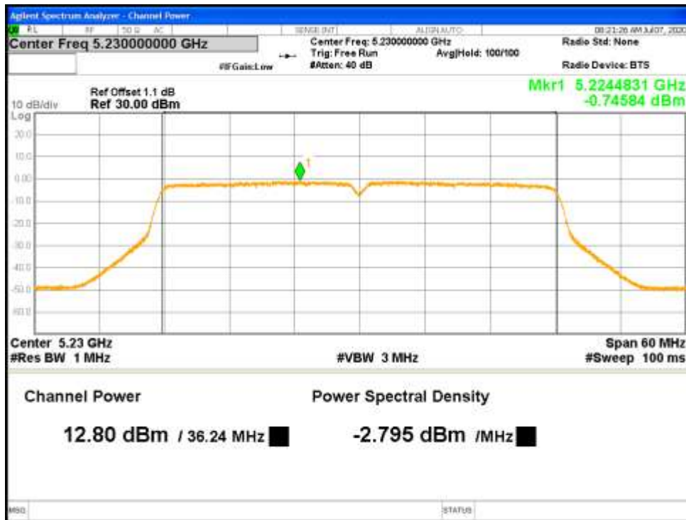
Figure 25: RSS Correlated Max Conducted Power-5230 MHz-802.11n-HT40-MCS0-Ch0
