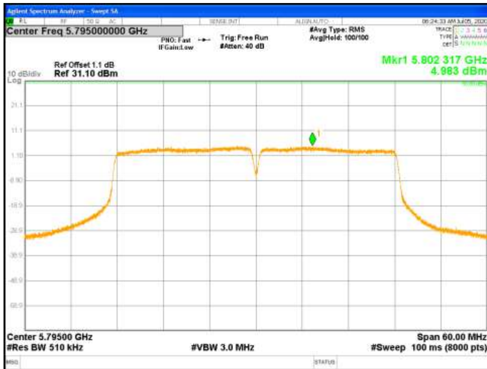
Figure 65: Correlated Power Spectral Density-5795 MHz-802.11n-HT40-MCS0-Ch0
