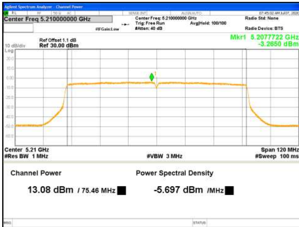
Figure 31: RSS Correlated Max Conducted Power-5210 MHz-802.11ac-VHT80-MCS0-Ch0
