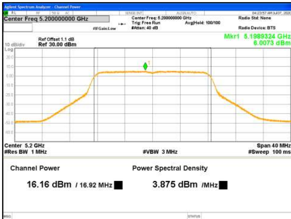
Figure 6: RSS Uncorrelated Max Conducted Power-5200 MHz-802.11a-6 Mbps-Ch1
