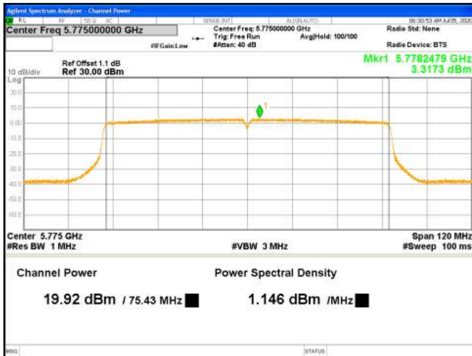
Figure 16: Uncorrelated Max Conducted Power-5775 MHz-802.11ac-VHT80-MCS0-Ch0
