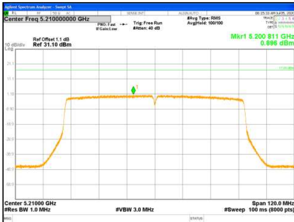
Figure 52: FCC Uncorrelated Power Spectral Density-5210 MHz-802.11ac-VHT80-MCS0-Ch0
