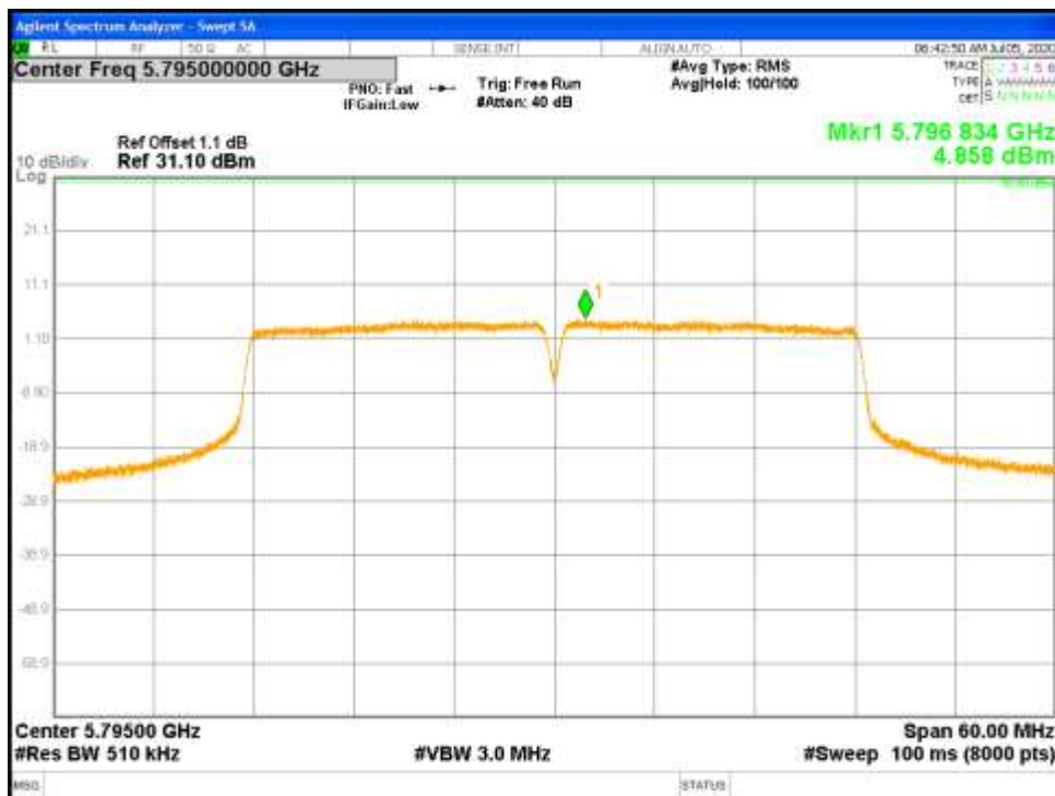
Figure 66: Correlated Power Spectral Density-5795 MHz-802.11n-HT40-MCS0-Ch1
