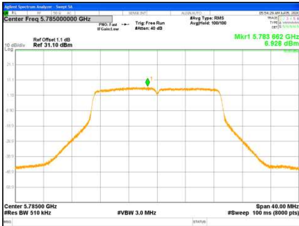
Figure 59: Correlated Power Spectral Density-5785 MHz-802.11n-HT20-MCS0-Ch0
