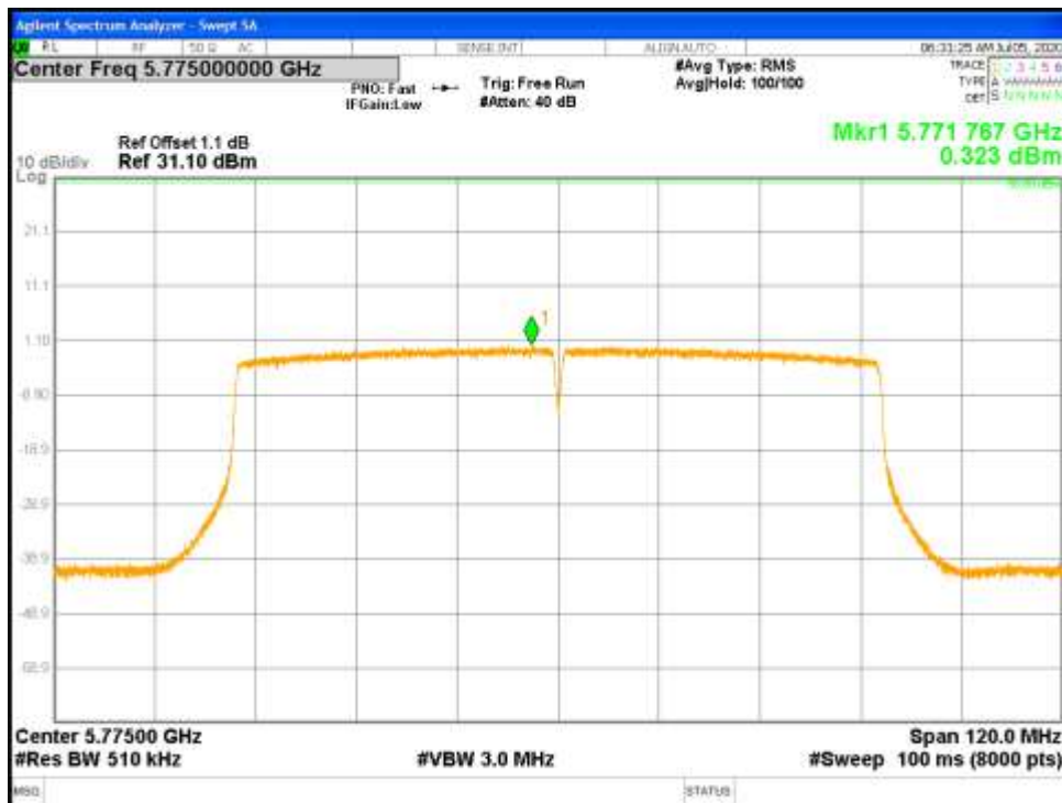
Figure 54: Uncorrelated Power Spectral Density-5775 MHz-802.11ac-VHT80-MCS0-Ch0
