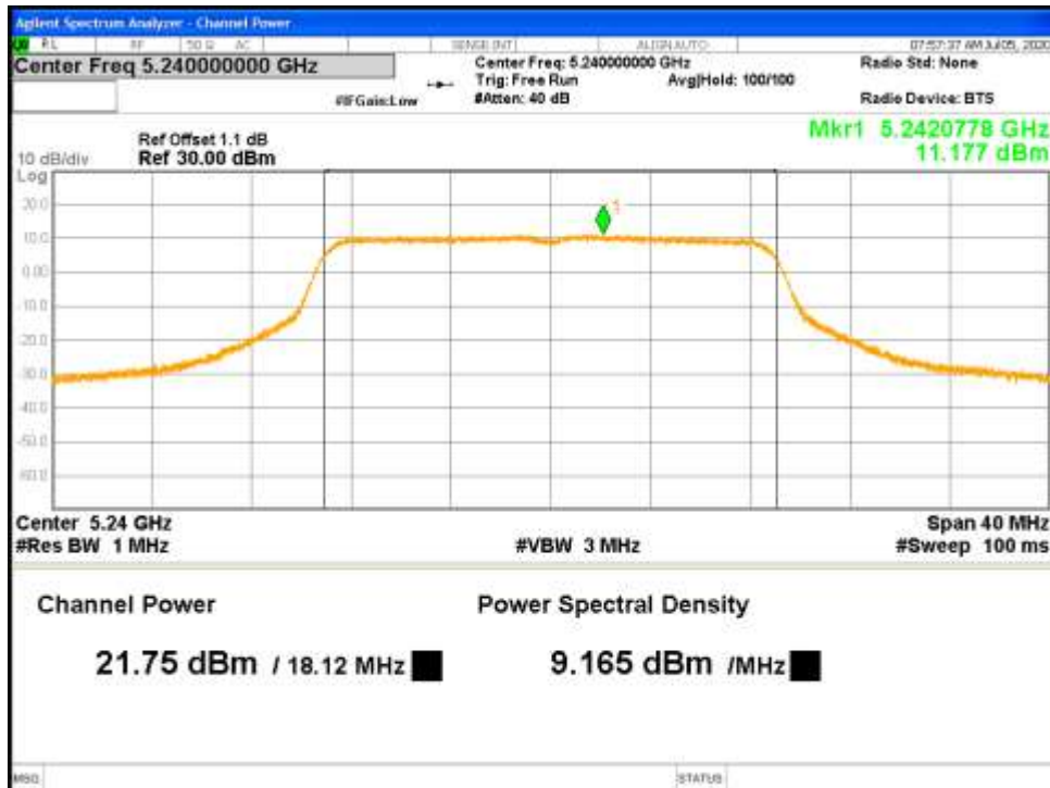
Figure 18: FCC Correlated Max Conducted Power-5240 MHz-802.11n-HT20-MCS0-Ch1
