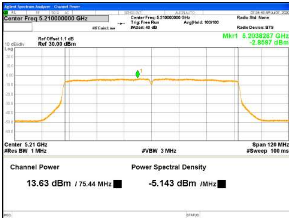
Figure 32: RSS Correlated Max Conducted Power-5210 MHz-802.11ac-VHT80-MCS0-Ch1
