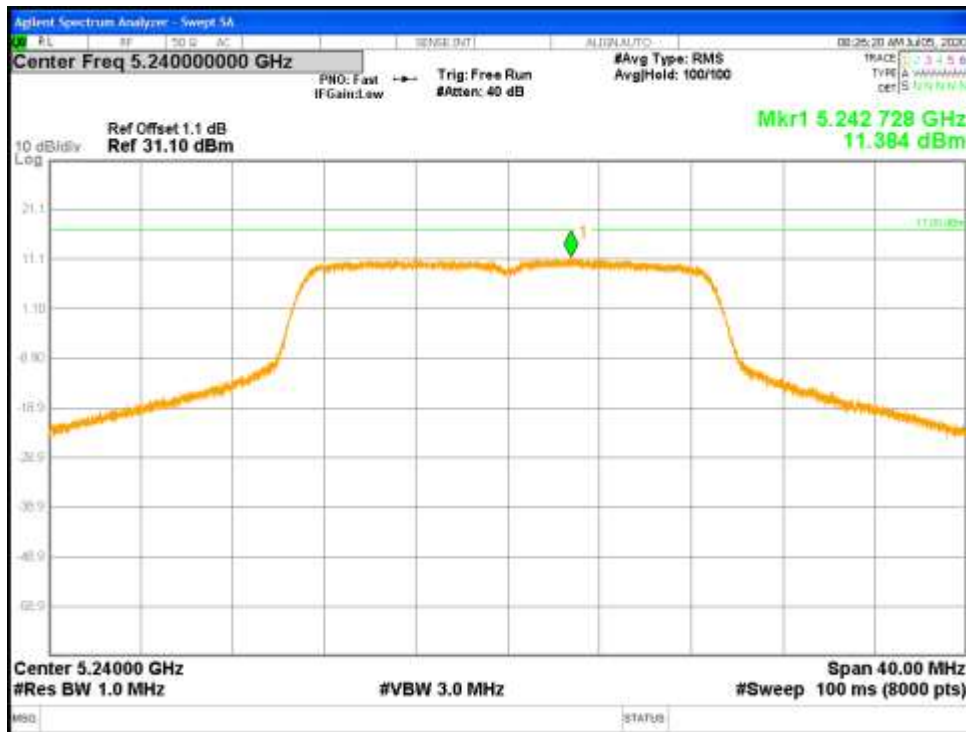
Figure 55: FCC Correlated Power Spectral Density-5240 MHz-802.11n-HT20-MCS0-Ch0
