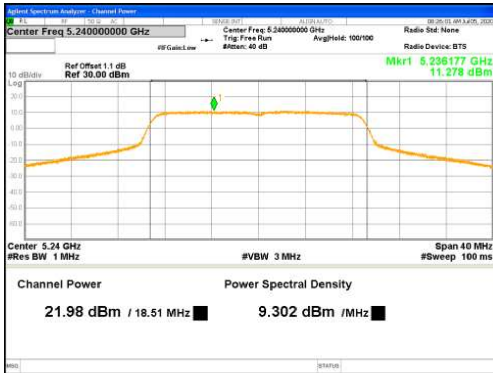
Figure 17: FCC Correlated Max Conducted Power-5240 MHz-802.11n-HT20-MCS0-Ch0
