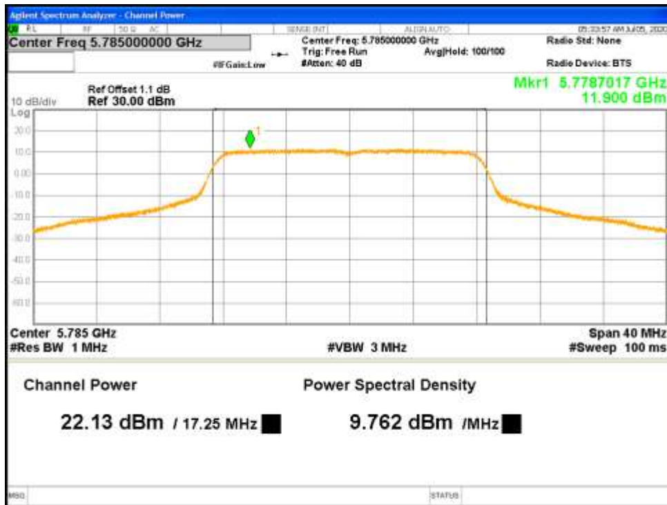
Figure 7: Uncorrelated Max Conducted Power-5785 MHz-802.11a-6 Mbps-Ch0
