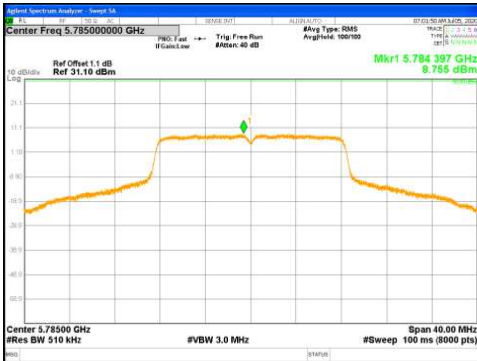
Figure 45: Uncorrelated Power Spectral Density-5785 MHz-802.11a-6 Mbps-Ch1
