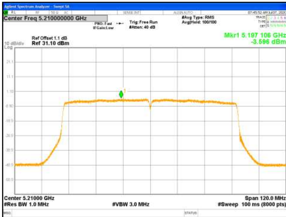
Figure 69: RSS Correlated Power Spectral Density-5210 MHz-802.11ac-VHT80-MCS0-Ch0
