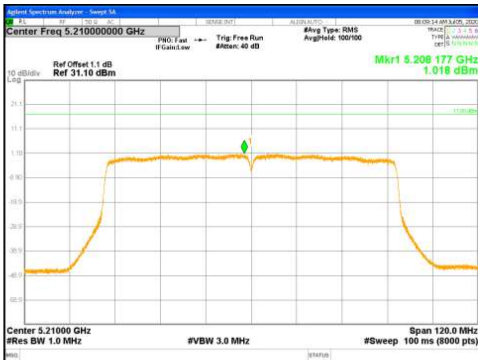
Figure 68: FCC Correlated Power Spectral Density-5210 MHz-802.11ac-VHT80-MCS0-Ch1
