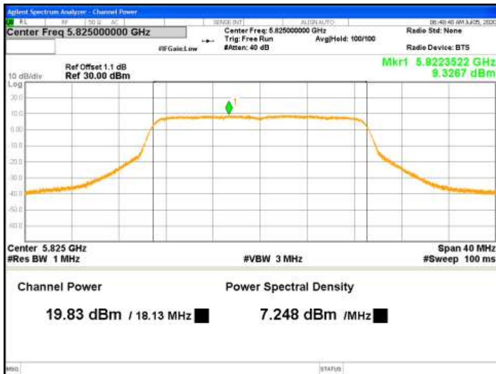
Figure 22: Correlated Max Conducted Power-5825 MHz-802.11n-HT20-MCS0-Ch1
