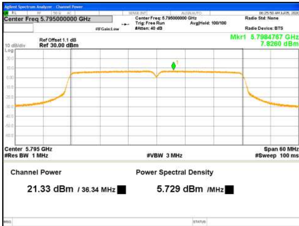
Figure 13: Uncorrelated Max Conducted Power-5795 MHz-802.11n-HT40-MCS0-Ch0
