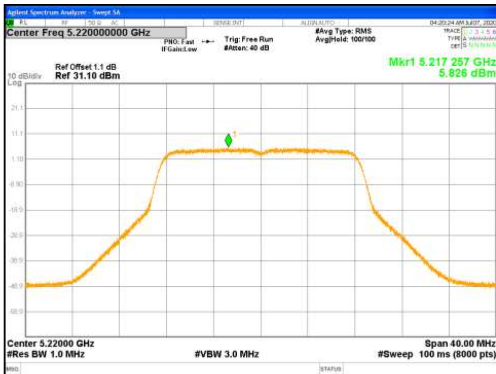
Figure 44: RSS Uncorrelated Power Spectral Density-5220 MHz-802.11a-6 Mbps-Ch1
