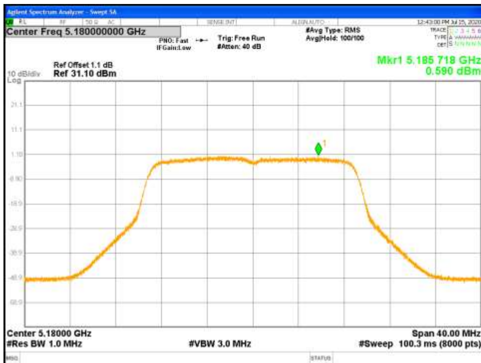
Figure 58: RSS Correlated Power Spectral Density-5180 MHz-802.11n-HT20-MCS0-Ch1
