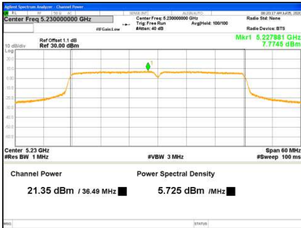
Figure 23: FCC Correlated Max Conducted Power-5230 MHz-802.11n-HT40-MCS0-Ch0
