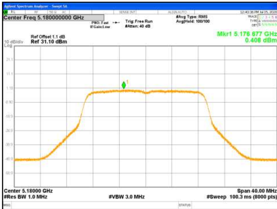
Figure 57: RSS Correlated Power Spectral Density-5180 MHz-802.11n-HT20-MCS0-Ch0
