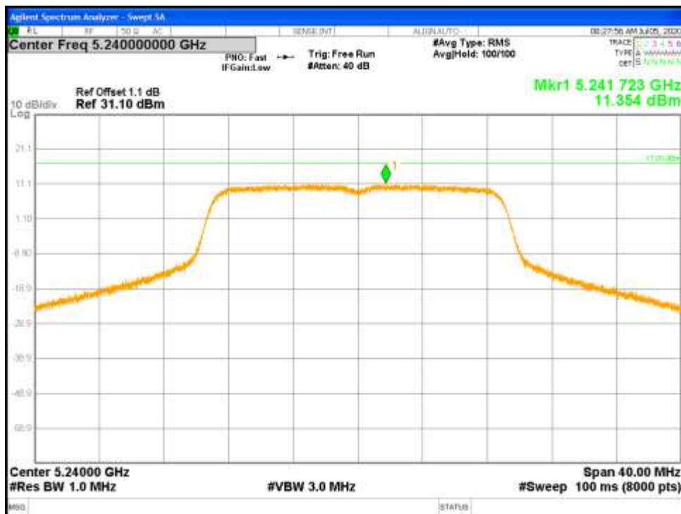
Figure 46: FCC Uncorrelated Power Spectral Density-5240 MHz-802.11n-HT20-MCS0-Ch0
