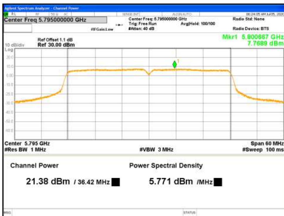
Figure 27: Correlated Max Conducted Power-5795 MHz-802.11n-HT40-MCS0-Ch0
