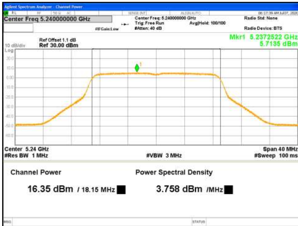
Figure 9: RSS Uncorrelated Max Conducted Power-5240 MHz-802.11n-HT20-MCS0-Ch0
