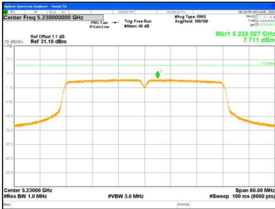
Figure 49: FCC Uncorrelated Power Spectral Density-5230 MHz-802.11n-HT40-MCS0-Ch0
