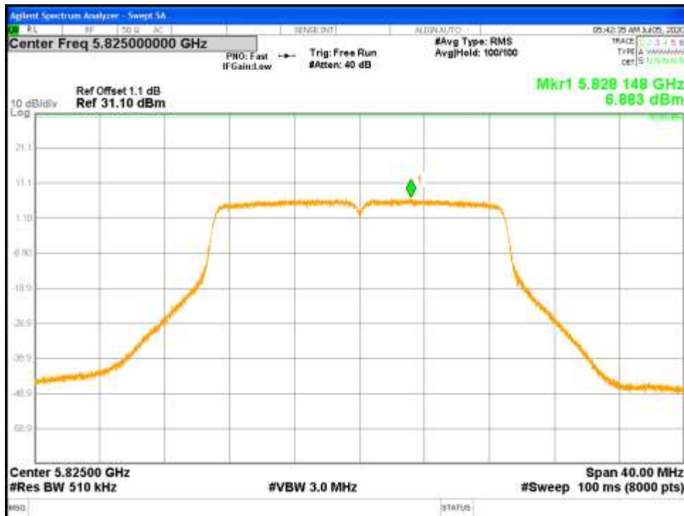
Figure 48: Uncorrelated Power Spectral Density-5825 MHz-802.11n-HT20-MCS0-Ch0
