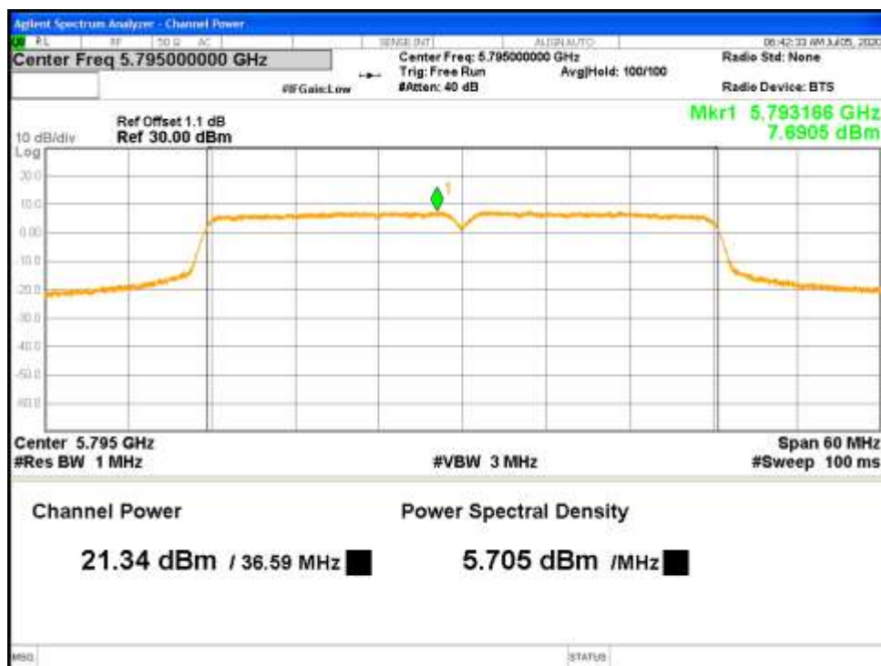
Figure 28: Correlated Max Conducted Power-5795 MHz-802.11n-HT40-MCS0-Ch1
