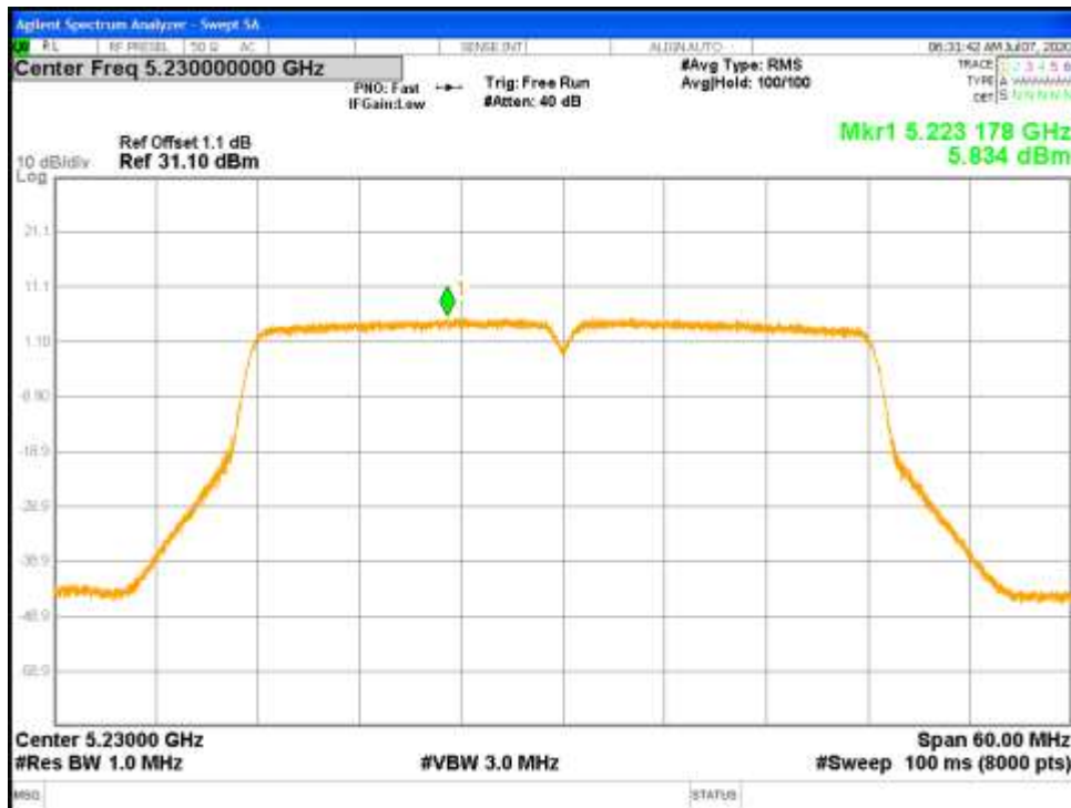
Figure 50: RSS Uncorrelated Power Spectral Density-5230 MHz-802.11n-HT40-MCS0-Ch0
