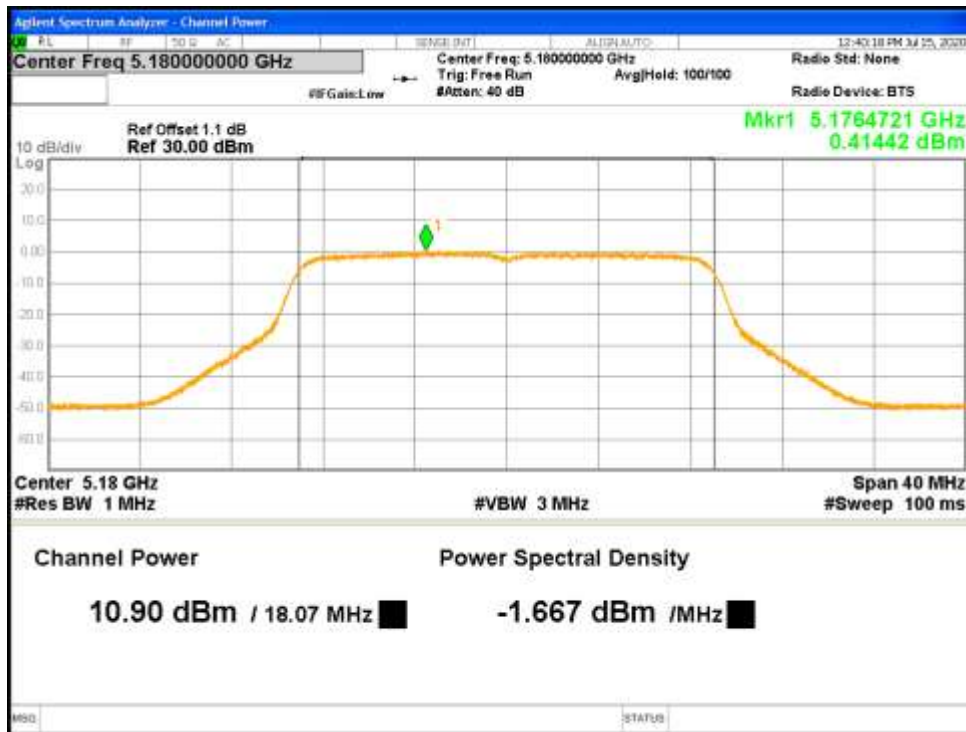
Figure 19: RSS Correlated Max Conducted Power-5180 MHz-802.11n-HT20-MCS0-Ch0
