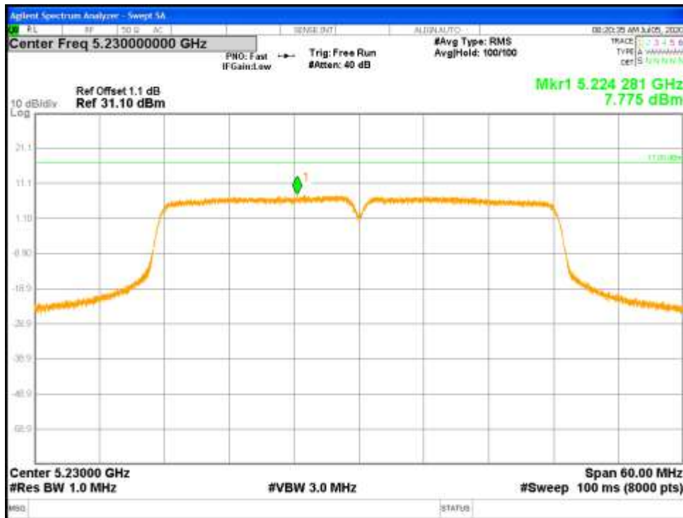
Figure 61: FCC Correlated Power Spectral Density-5230 MHz-802.11n-HT40-MCS0-Ch0
