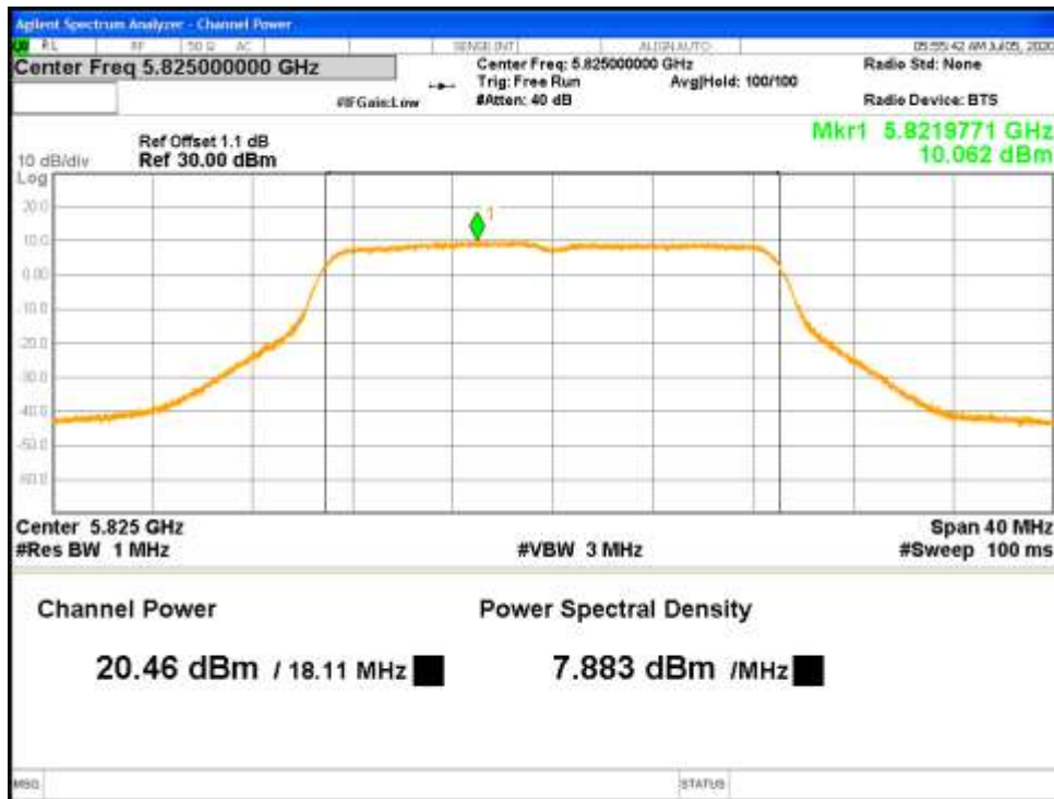
Figure 21: Correlated Max Conducted Power-5825 MHz-802.11n-HT20-MCS0-Ch0
