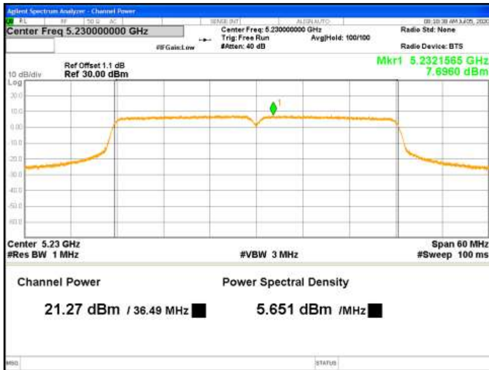
Figure 11: FCC Uncorrelated Max Conducted Power-5230 MHz-802.11n-HT40-MCS0-Ch0
