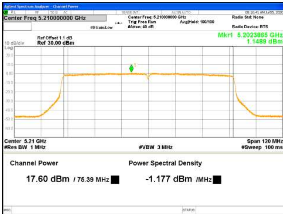
Figure 29: FCC Correlated Max Conducted Power-5210 MHz-802.11ac-VHT80-MCS0-Ch0
