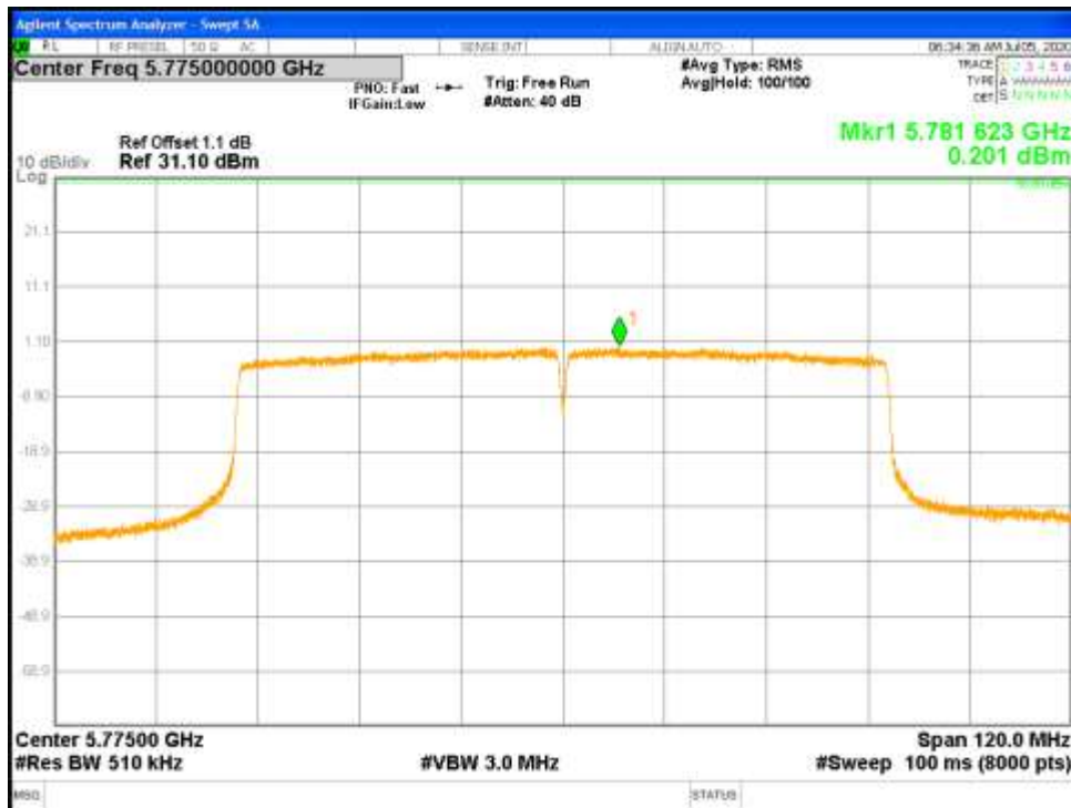
Figure 72: Correlated Power Spectral Density-5775 MHz-802.11ac-VHT80-MCS0-Ch1
