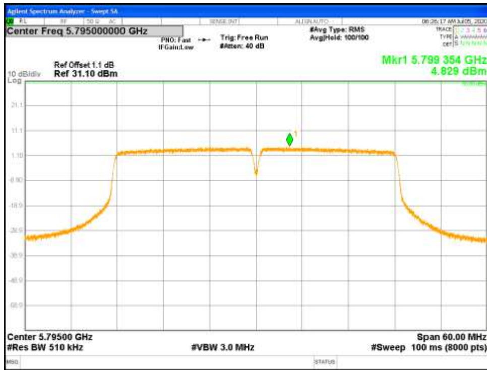
Figure 51: Uncorrelated Power Spectral Density-5795 MHz-802.11n-HT40-MCS0-Ch0
