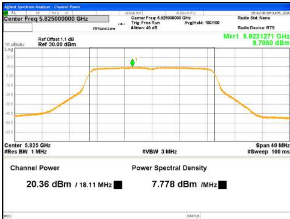
Figure 10: Uncorrelated Max Conducted Power-5825 MHz-802.11n-HT20-MCS0-Ch0
