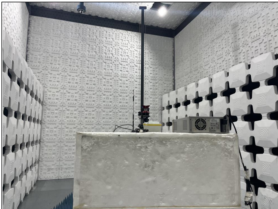
Radiated emission test: Frequency Range < 9KHz- 30MHz >
