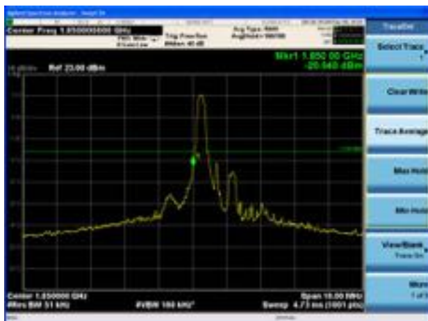
LTE Band 25 1.4MHz 16QAM 100%RB CH-Low
