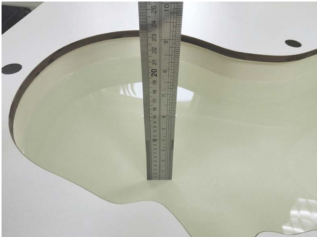
Liquid depth in the head Phantom (1900 MHz, 15.3cm depth)
