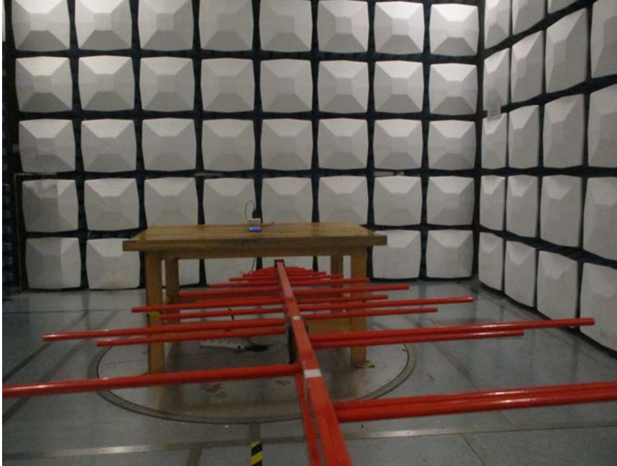
Radiated Emission View (Below 1GHz)
