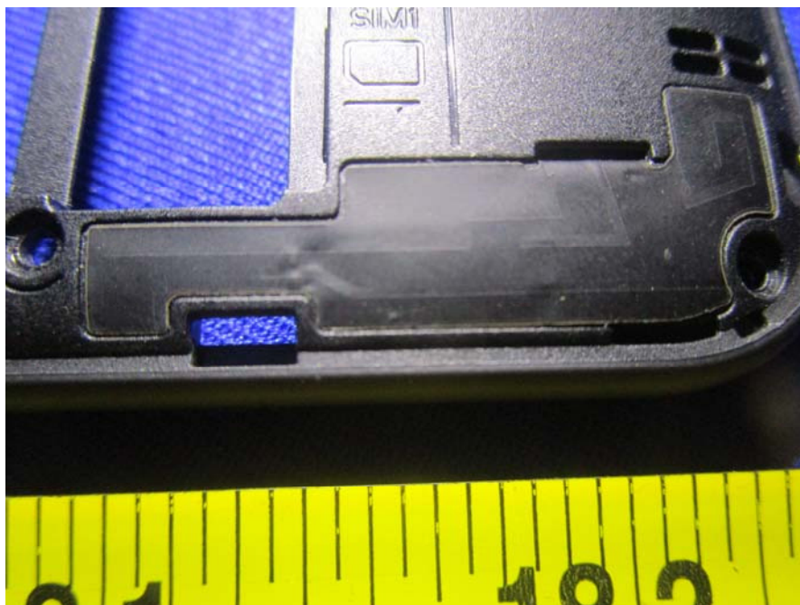
EUT –BT & WIFI & GPS Antenna View
