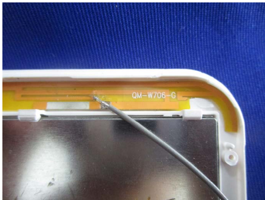
EUT – GSM&WCDMA Antenna View
