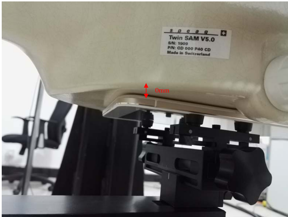
Body-worn Back Setup Photo (0mm)
