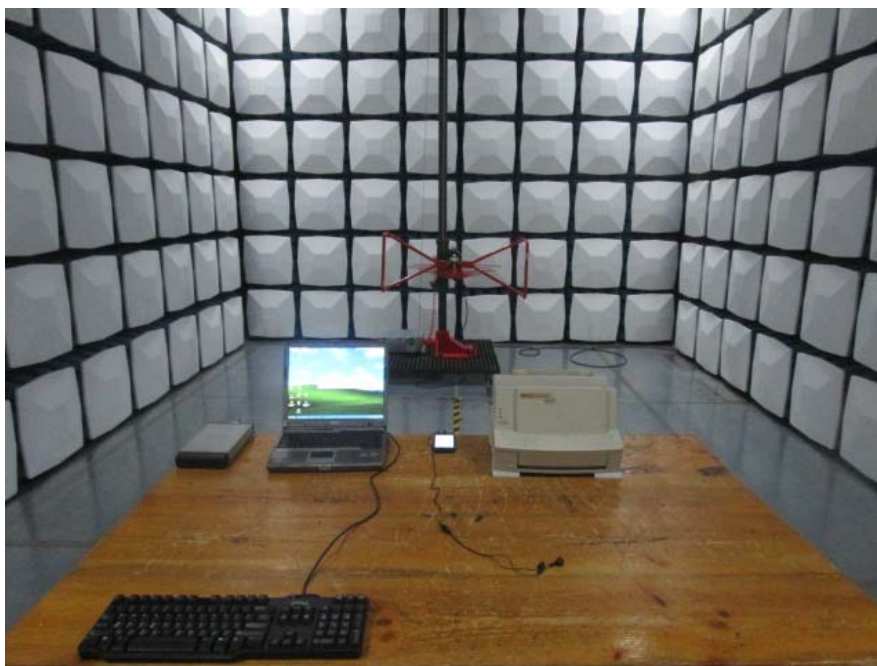
Radiated Emissions –Front View (Below 1GHz)
