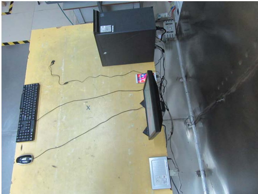
Conducted Emissions - Side View
